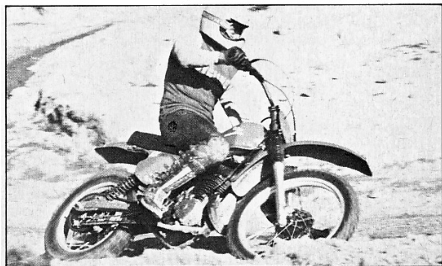
Our favorite part of the "R" model . . . engine is powerful, has surprisingly wide powerband. Pipe is well tucked in. Note left-side kickstarter, unusual for Japanese bikes. Steel tank holds 2.2 gallons.
