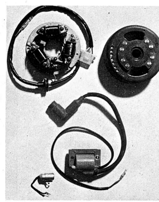
In order to give the Honda the extra tractability desert riding requires, the MT ignition with its heavier flywheel was installed. It, too, flips right in without modification.
