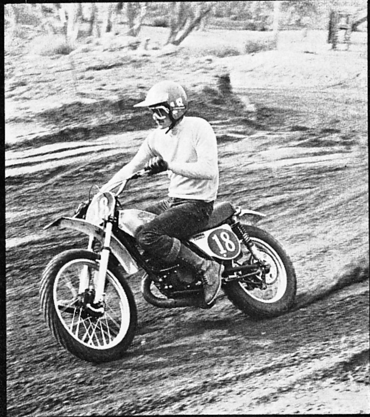
High volume exhaust pipe is an important factor in power package. Kick starter tucks in out of way. Entire engine weighs but 67 lb.
