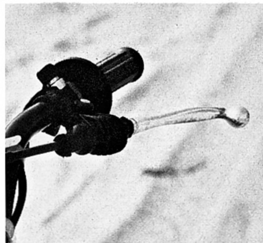
Good detailing, like rubber covers and nylon ties, can be found all over the 125.
