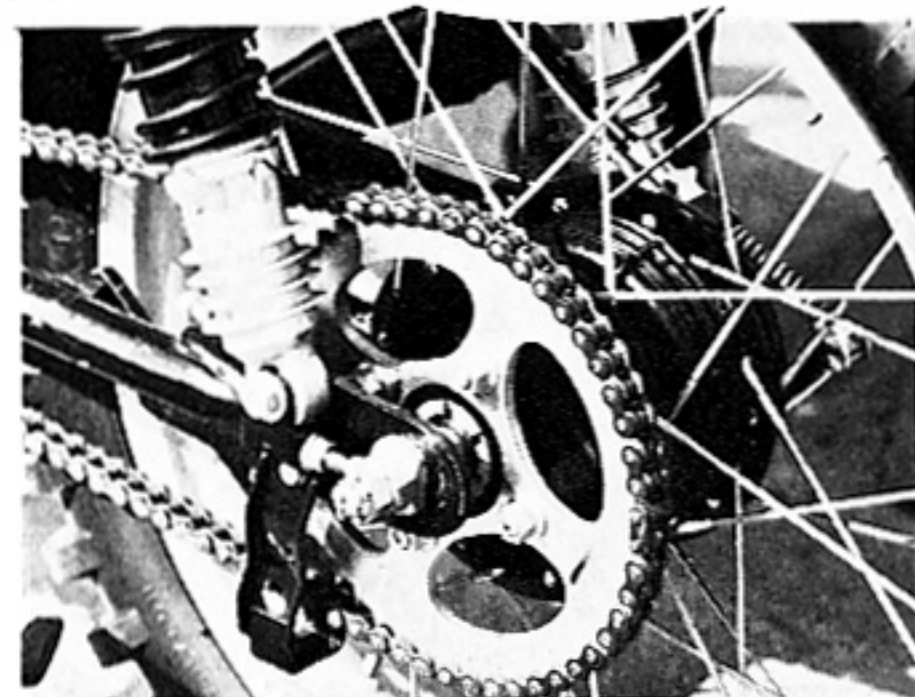
Small improvements for '75. Bigger sprocket bolts cure shearing problem of past. Chain guide is wimpy. Kickstand hangs out too far; needs grinding of tab to tuck in properly.
