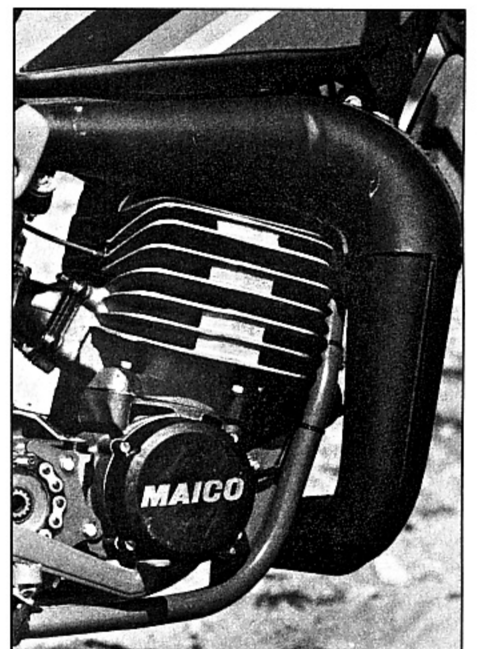
Although more violent than in the past, the Maico is still a broad mid-range powerband. Maico's 86.5mm bore and 83mm stroke reed-valve motor is fed by a 40mm Bing.
