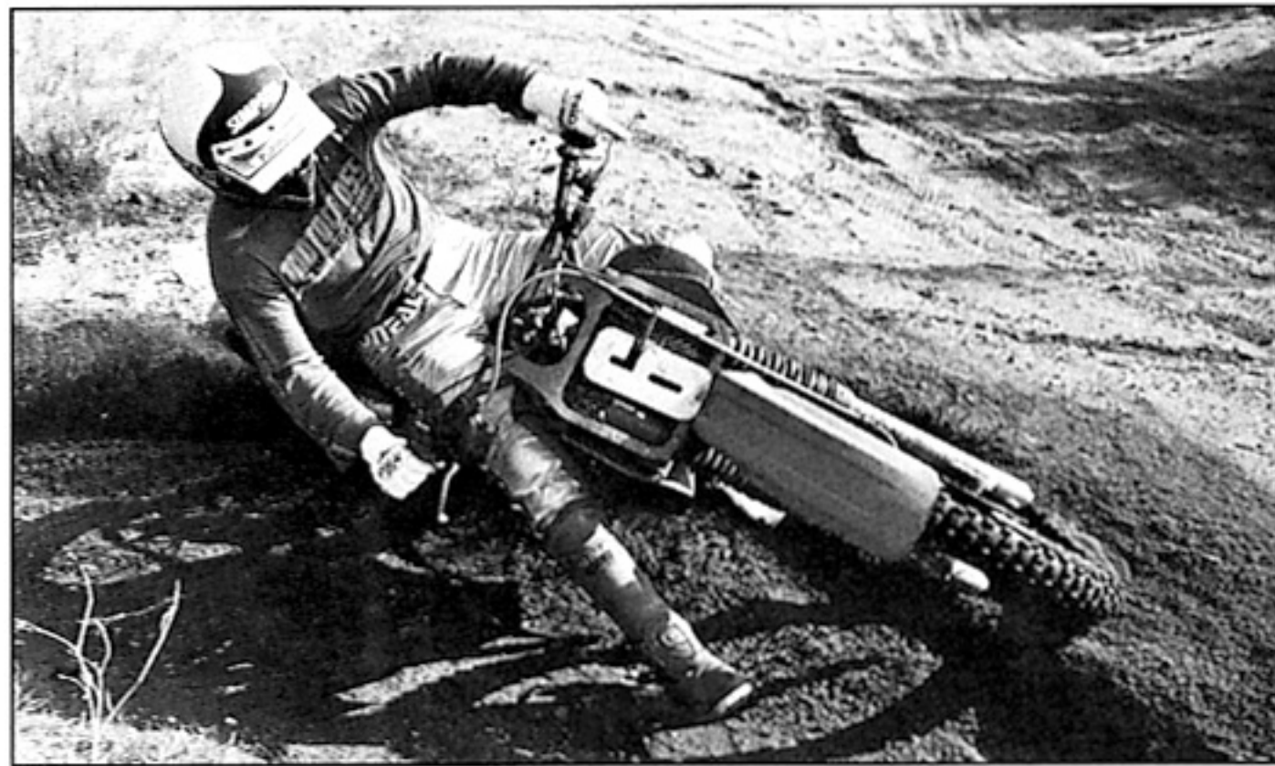
Kawasaki suffered from poor spring rates, hampering its handling; all of the Kayaba-forked bikes showed similar symptoms.
