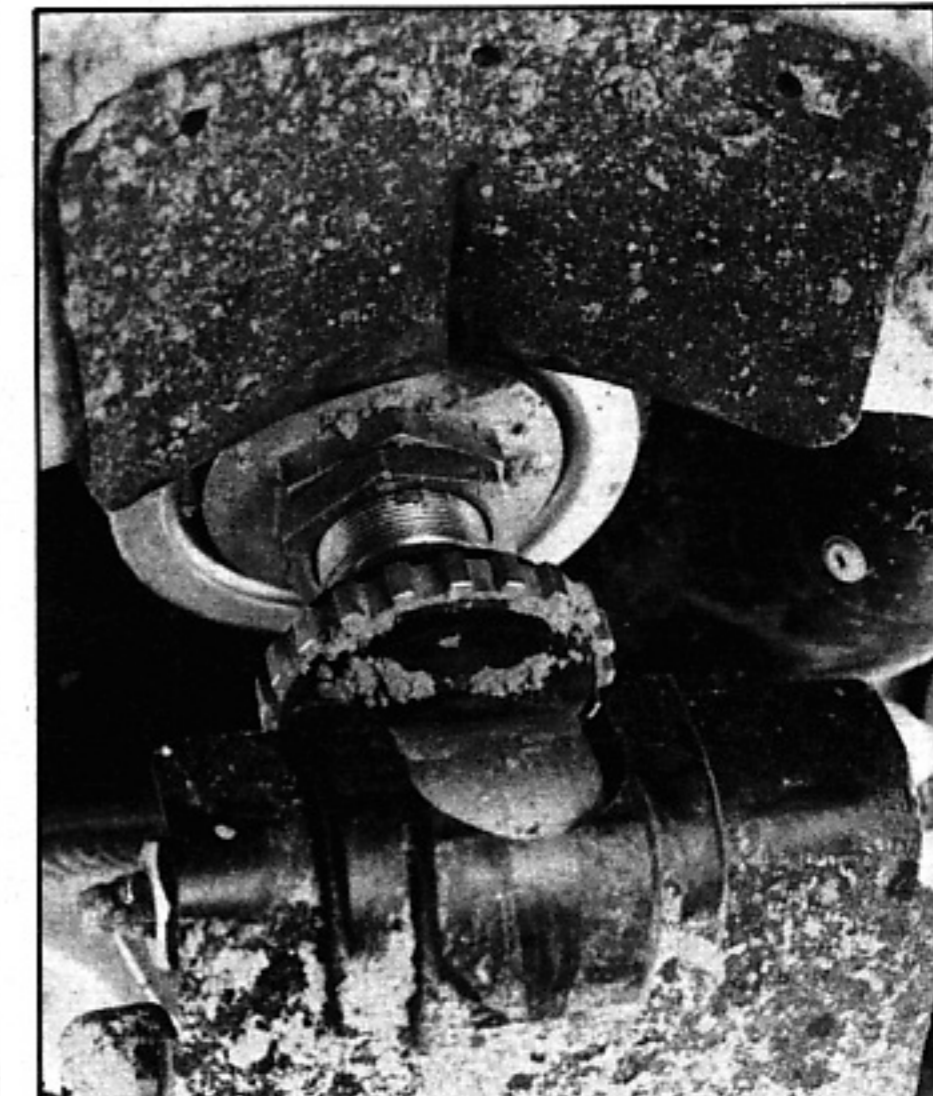
Zerk fitting and a larger, more-easily-accessible damping adjuster are nice touches on the Yamaha.
