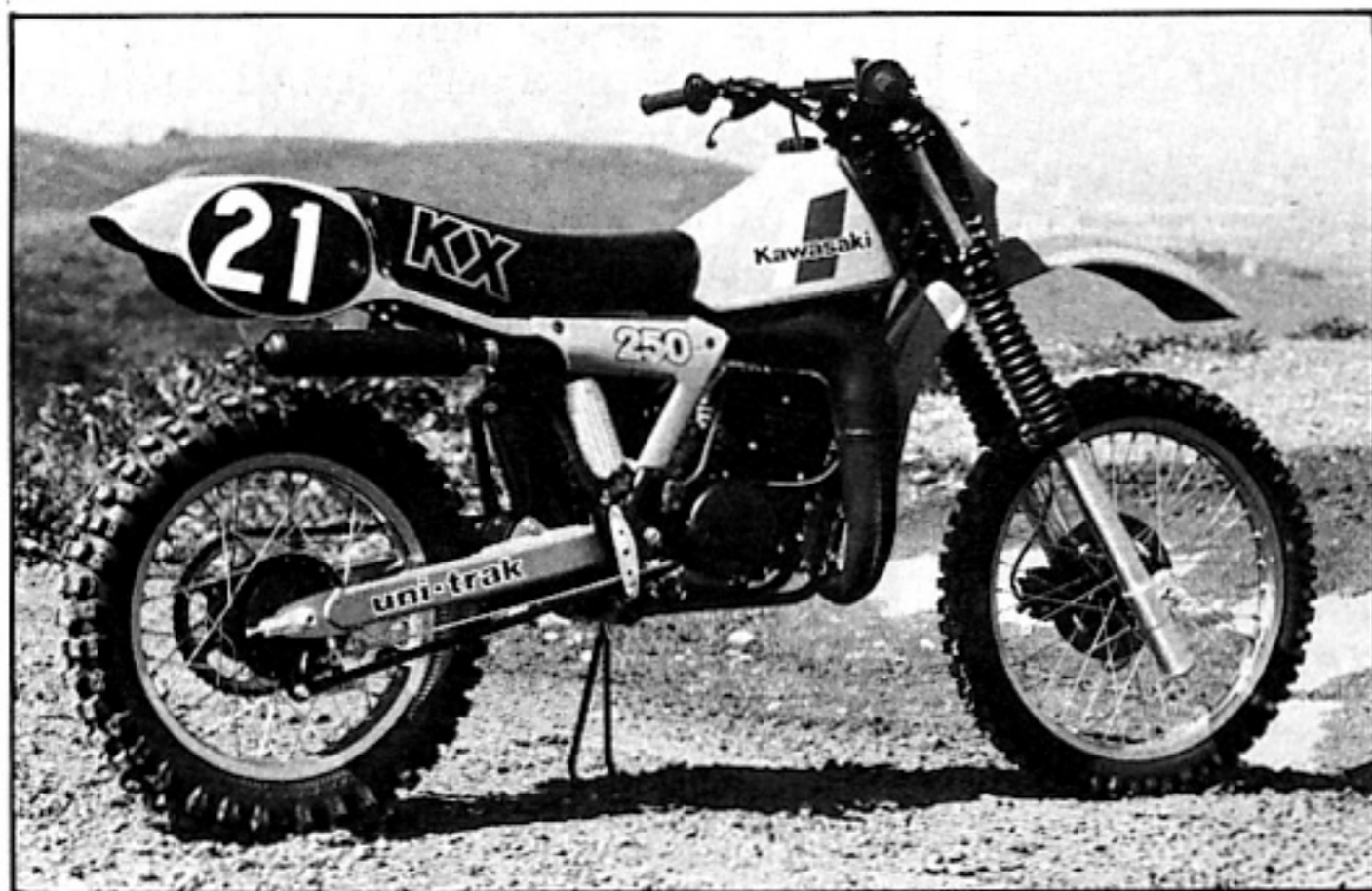
Kawasaki made a lightweight, air-cooled, disc-braked 250 that needs some subtle suspension care to bring it up to snuff.
