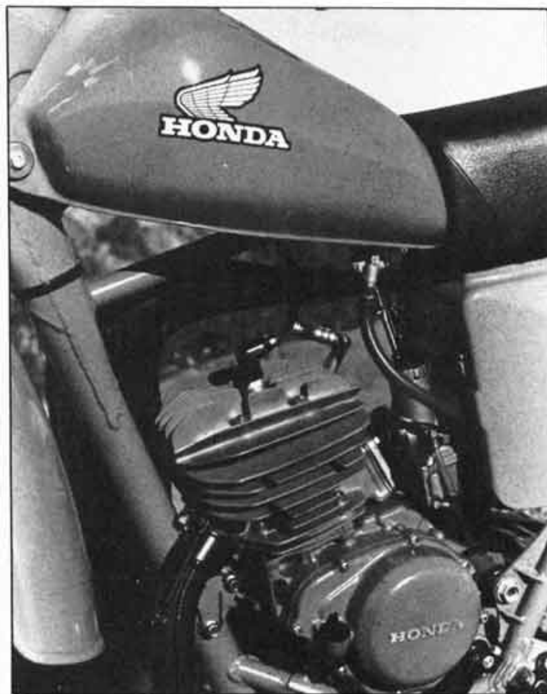
The gas tank is aluminum, so the decals won't be falling off like you know who. The reed-valved red engine has an abundance of torque and a broad, mellow powerband.
