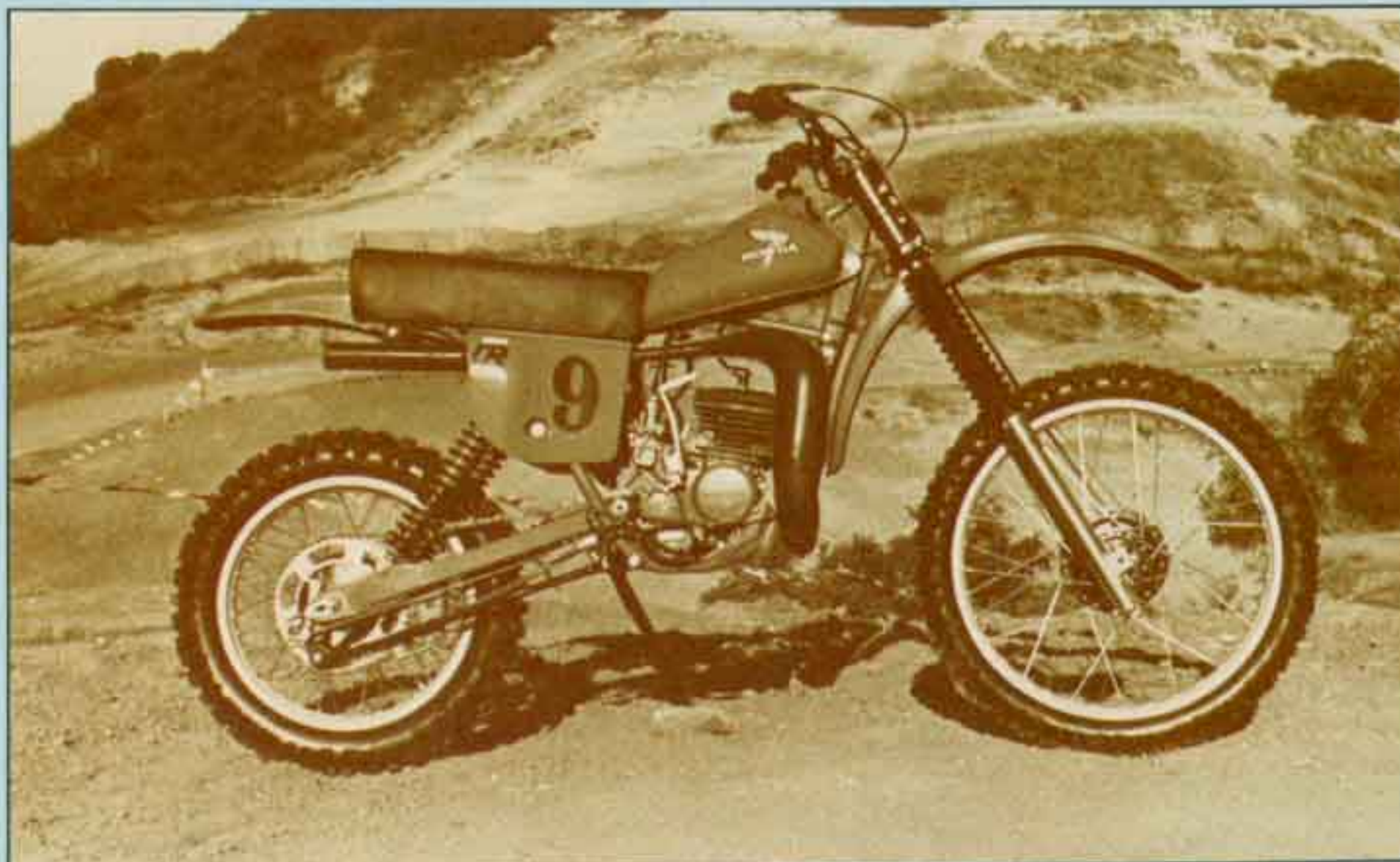
The front end is hoisted up on a 23-inch front wheel that gives the CR125R a skyscraper look.
