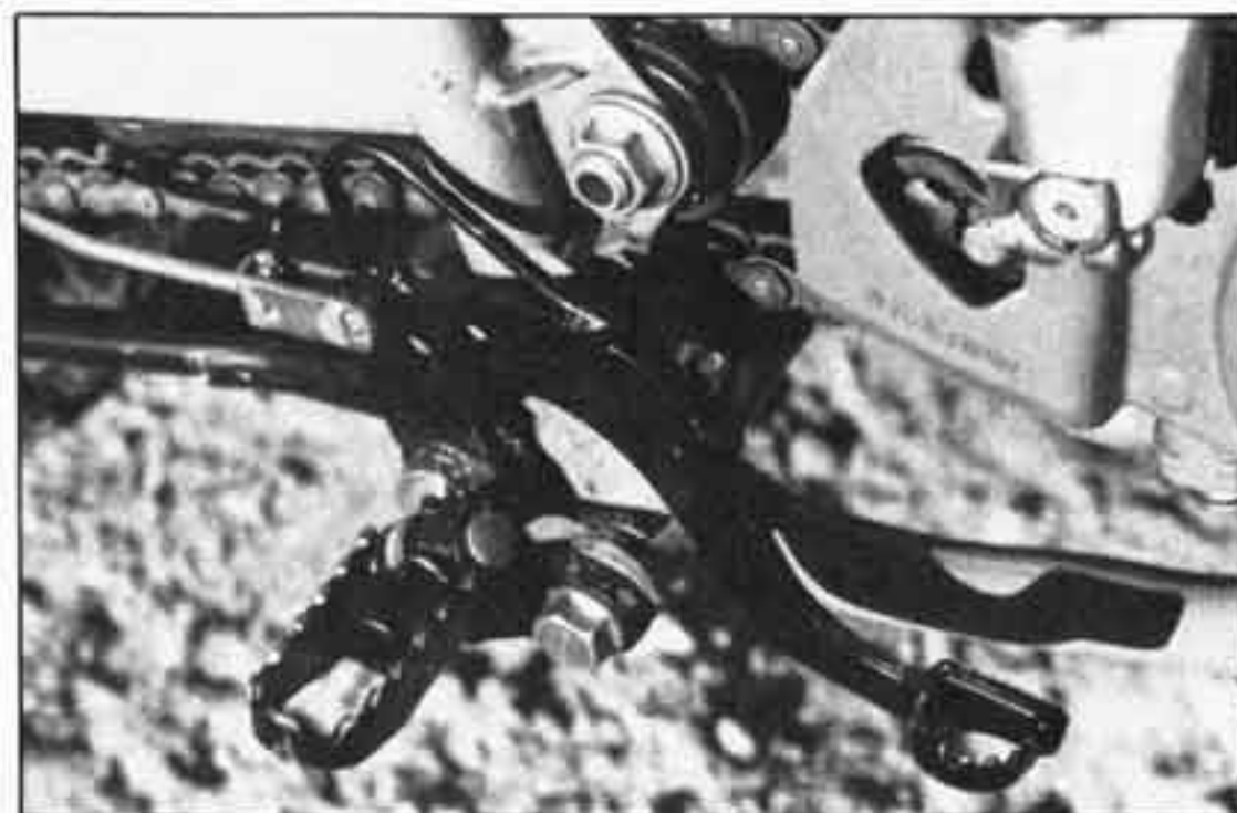
The footpegs are wimpy and will bend rearward. The coat hanger-type boot guard works best when it is tapped closer to the frame.
