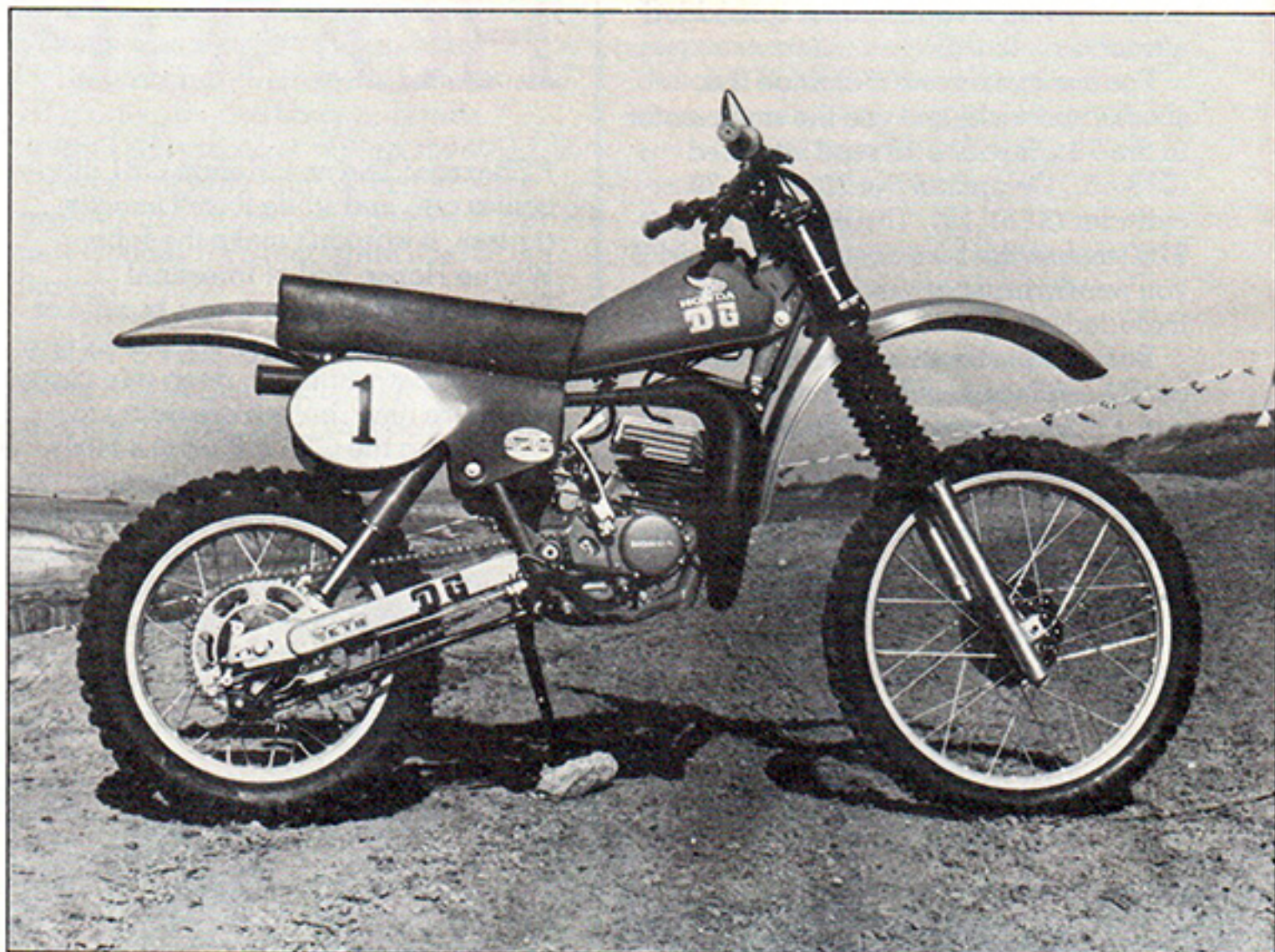
Kayaba's new single-rate air shocks look like Fox's without the fins. Paired with the aluminum swingarm they straighten out the Honda hop.
