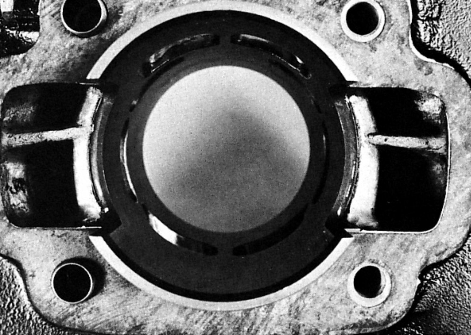
Some obvious features of the porting in the cylinder are the staggered inlet, canted roof on the rearward transfer ports, and the upper radius on the exhaust port which is bridged.
