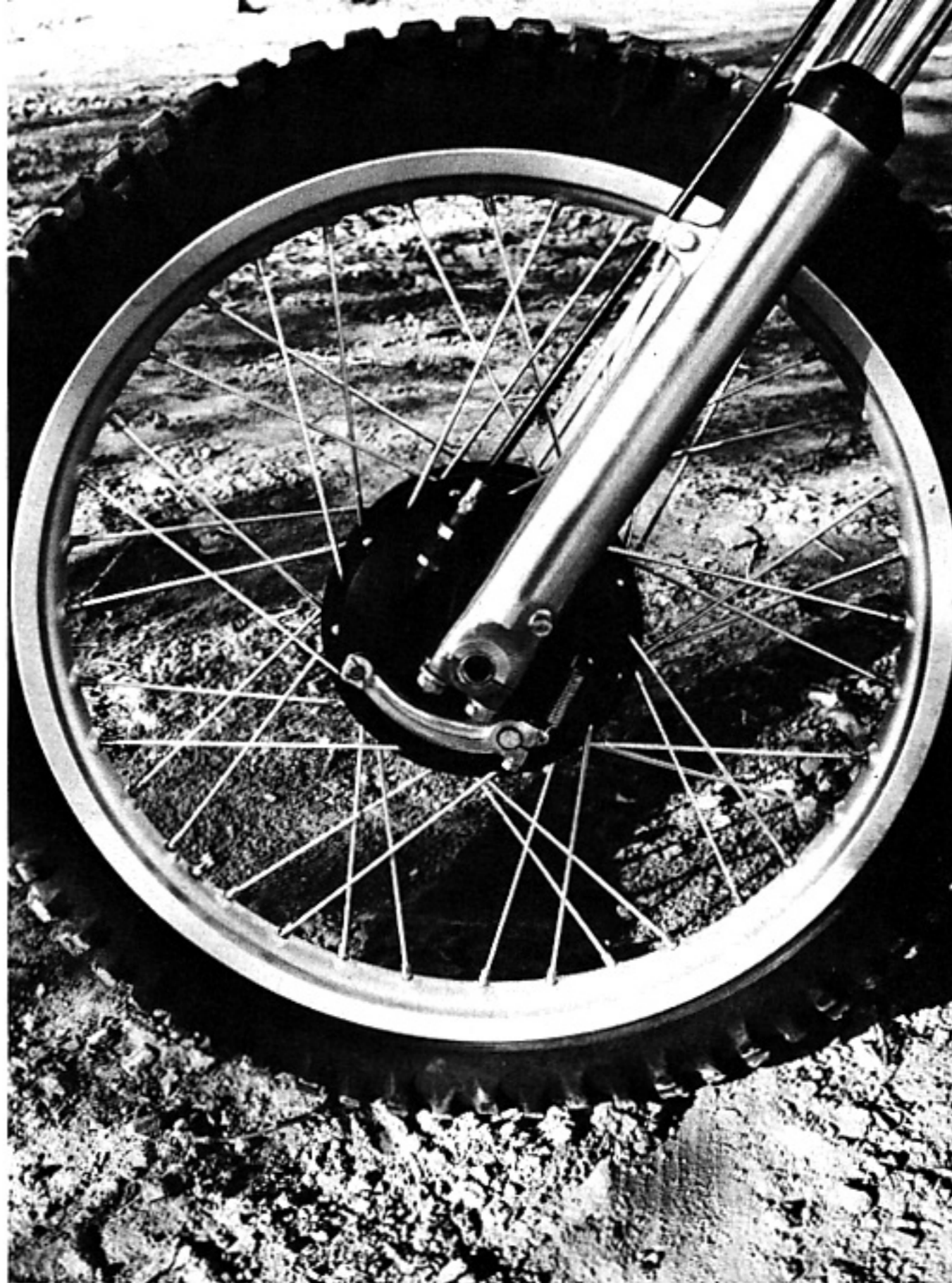
Sliders are machined from aluminum billets for light unsprung weight and extra strength. Note external return spring on the brake arm.
