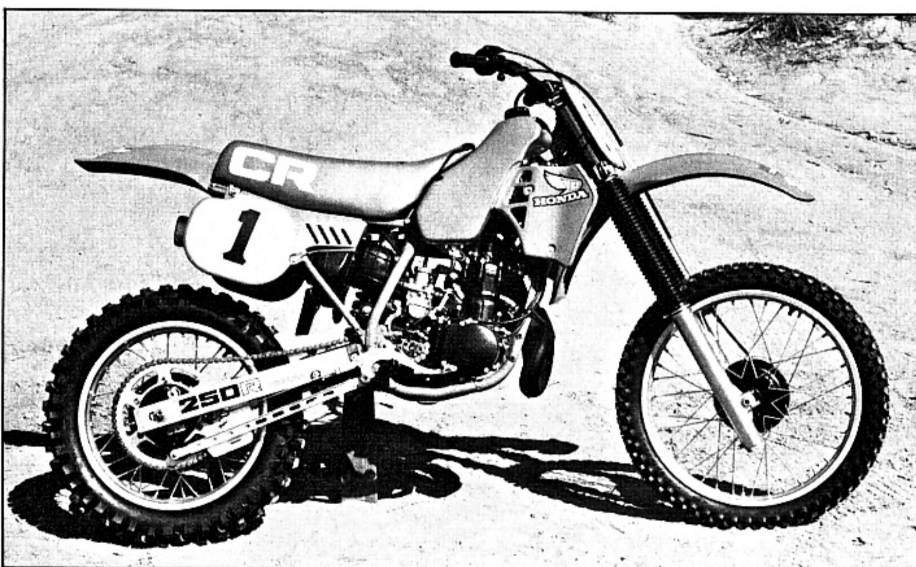
Superior front brake was a one-finger-stopper, due to the double-leading shoe arrangement.
