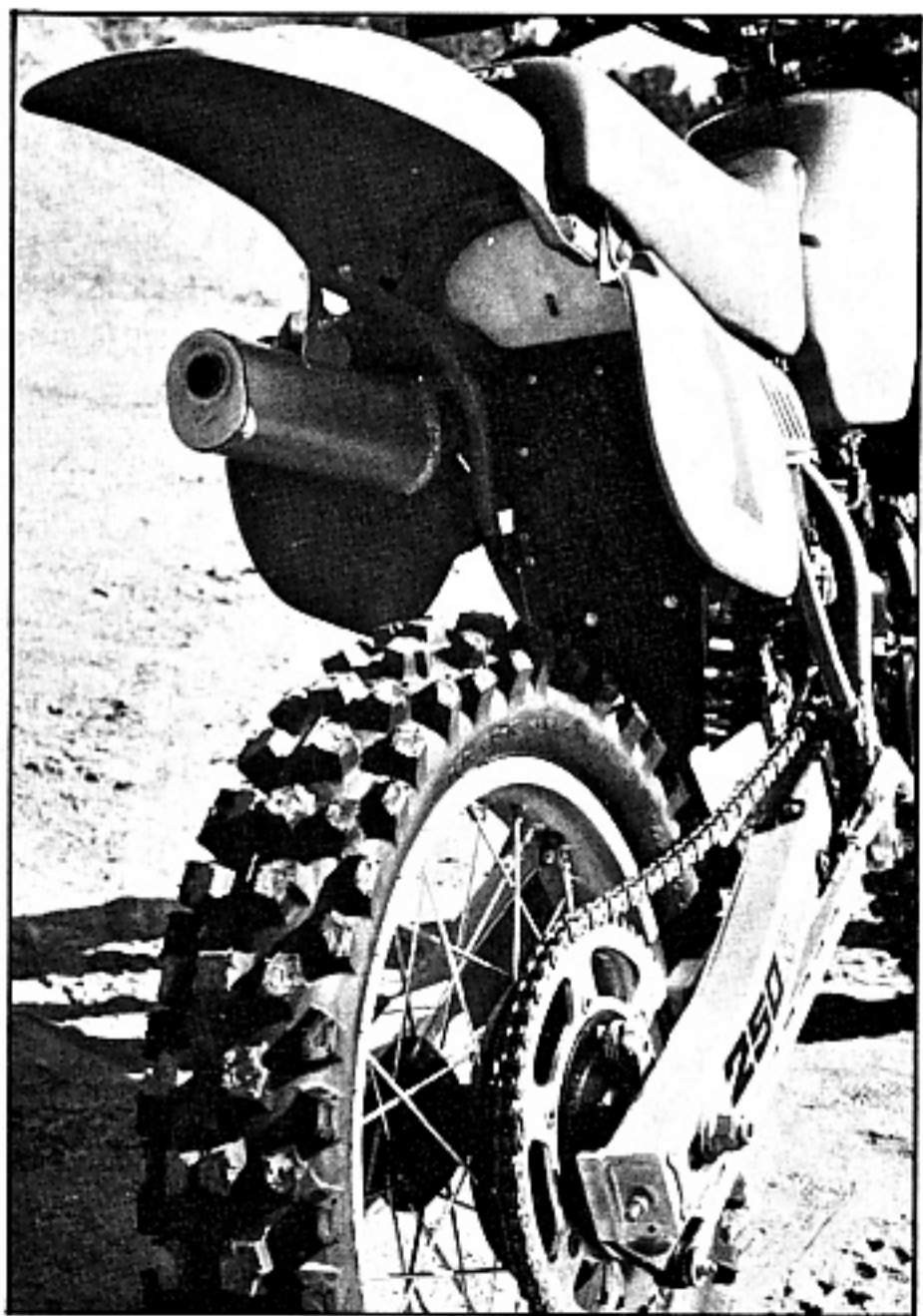
Worm's eye view of the rear end shows adequate clearance for the long travel. Box swingarm does not flex. Oval aluminum muffer gives good volume without taking up lateral space. Bike is extremely narrow.
