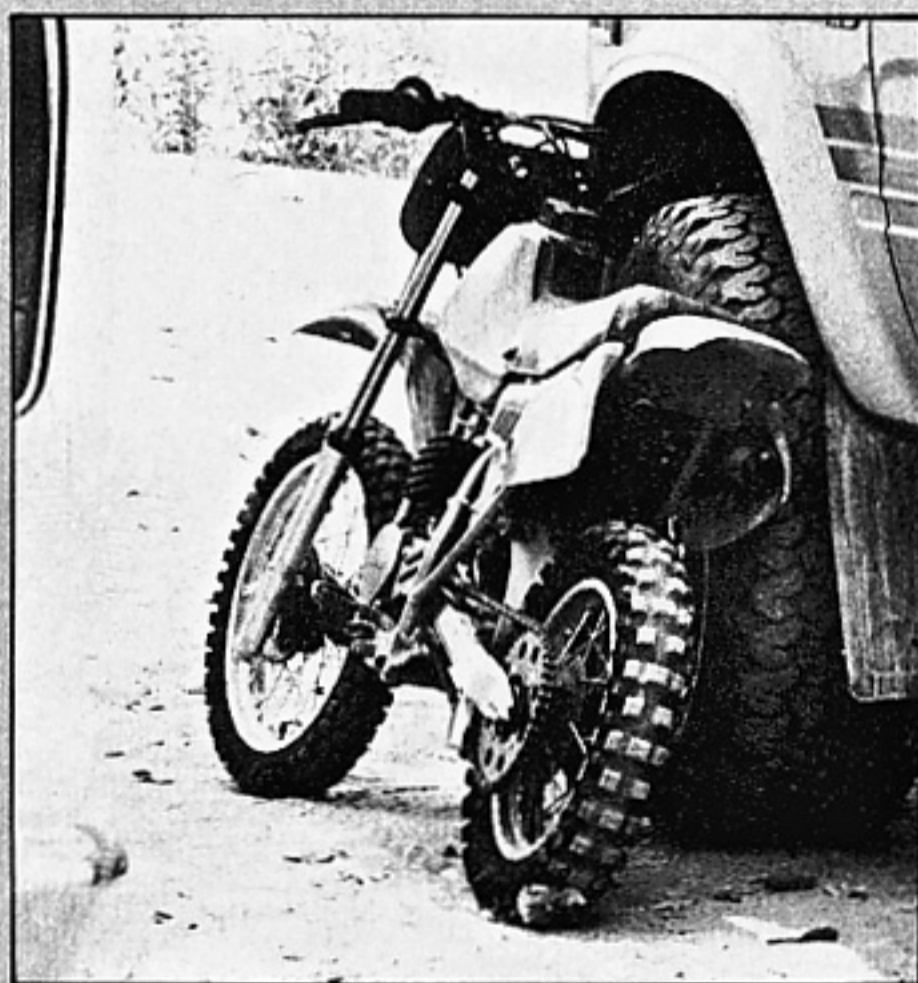
Here's a rear angle view of the 60. A safety seat and worklike tank can be seen, as well as a Pro-Link rear suspension. The engine is air-cooled and seems like a basic, ordinary two-stroke; we didn't ride the bike, so we have no guesses on performance.
