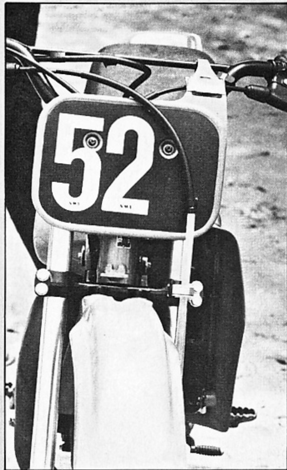
Seen from the front, the radiator sticks out a bit less than a typical Suzuki set-up. Numberplate will probably be different on the production version, with more protection down low and slots for air passage.
