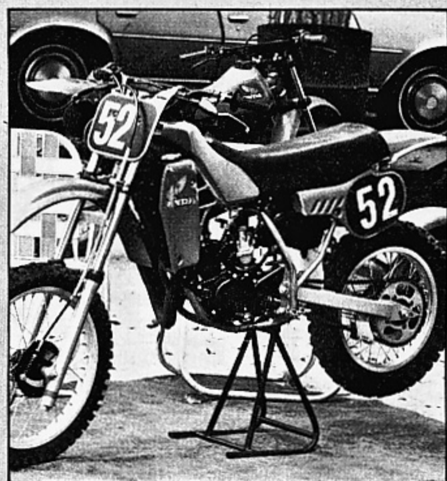
Here's another angle that shows the radiator placement. Very heavy gussets can be seen on the steering head, with lots of holes for weight reduction. The tires are new two-ply high-performance mini specials and appear to be Bridgestones.
