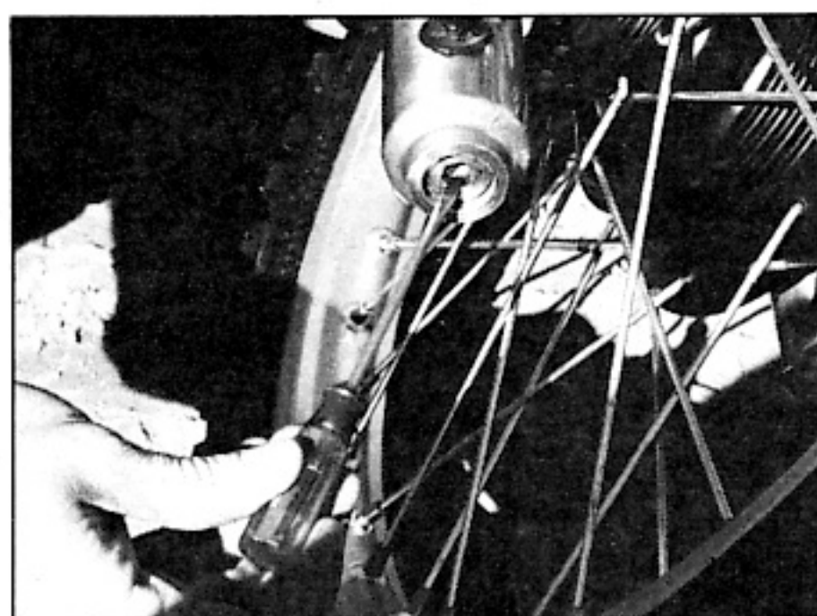
To adjust the compression damping on the forks, all you have to do is remove a rubber plug and twist a screwdriver. It's a lot easier with the bike on its side.
