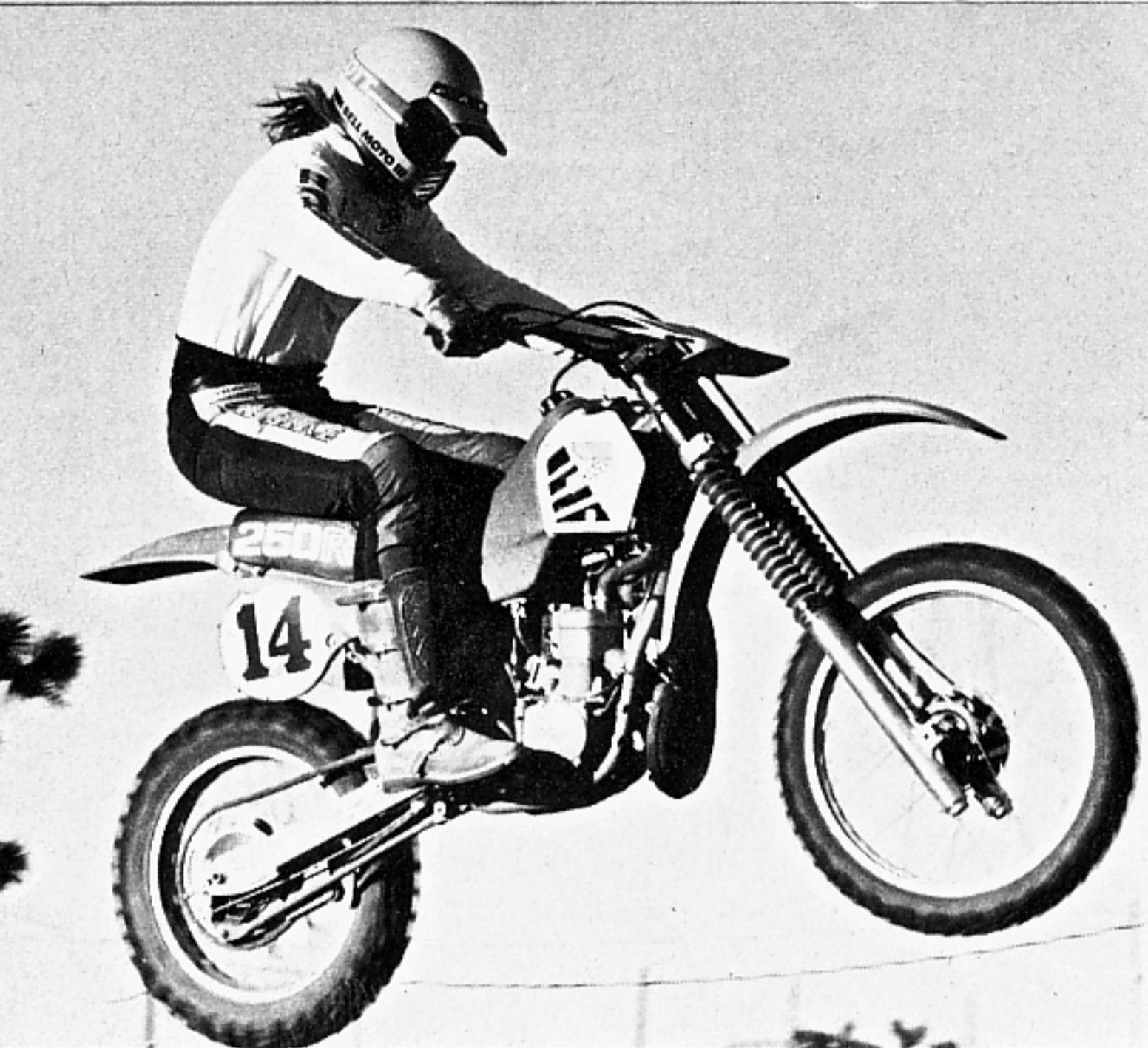
Twin radiators are very light and mount on each side of the tank. Plastic scoop on sides directs air to radiators; they fold in easily if the bike is dropped, then spring back into shape.
