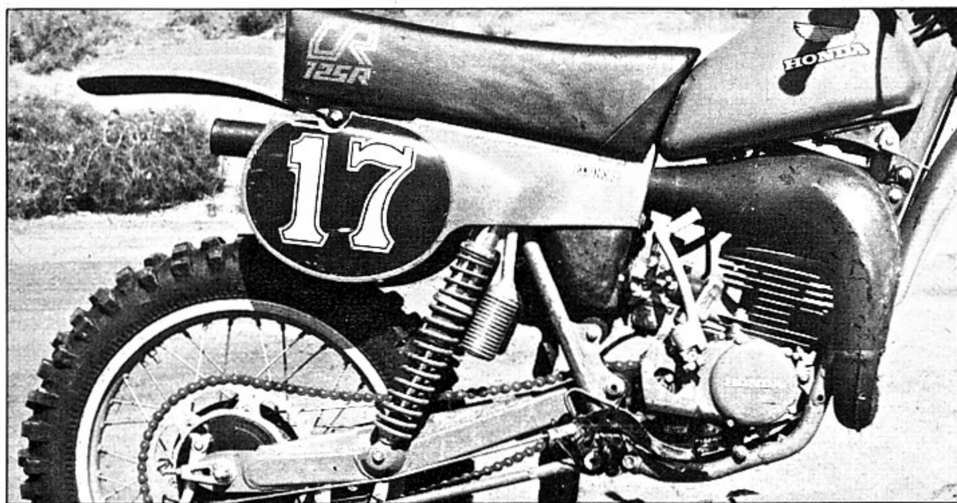
A banana-type swingarm went on the '80 Elsinore, to keep the seat height down after the addition of new Showa reservoir shocks.
