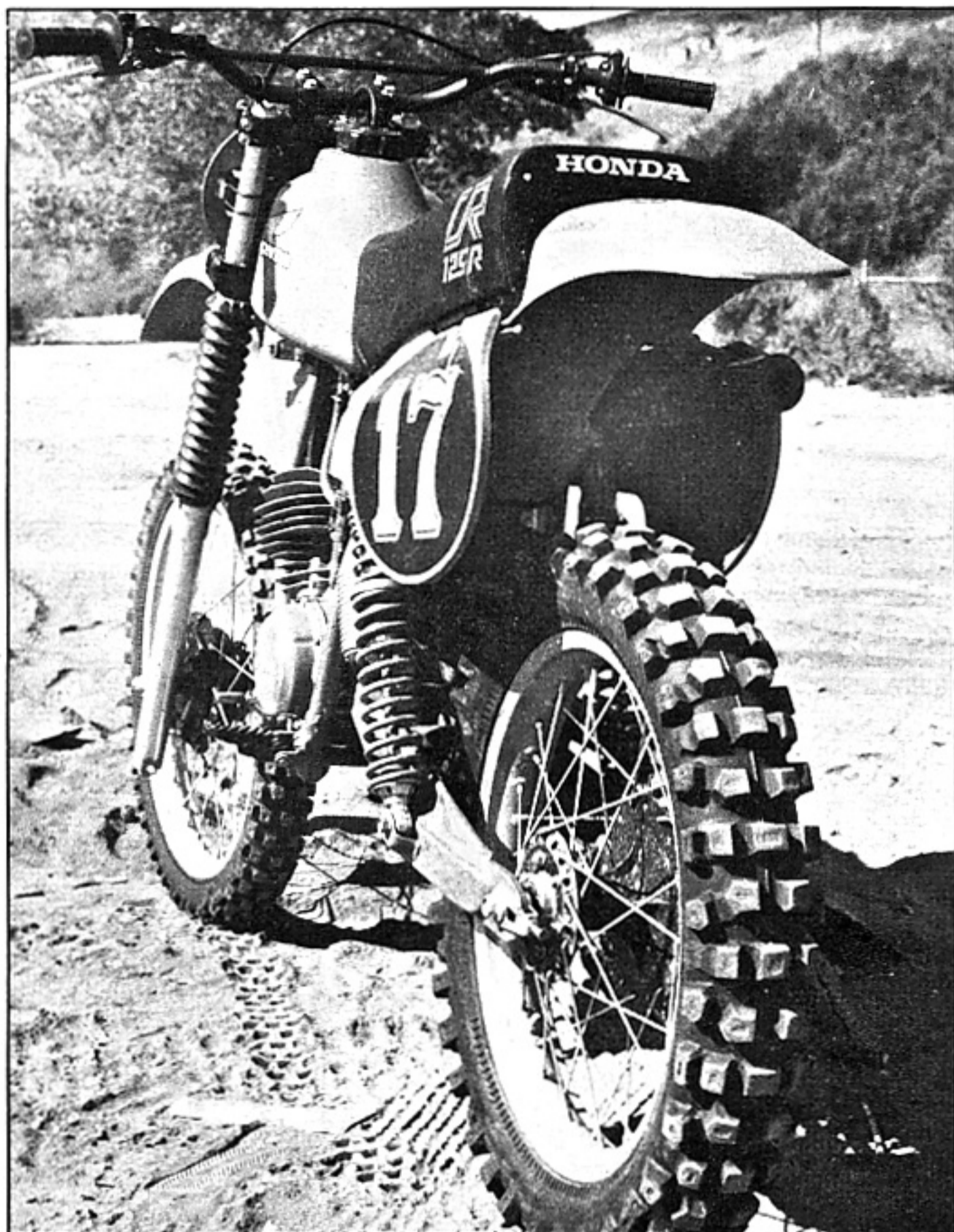
Last year's grim Claw-Action tires have been replaced with decent knobbies front and rear.
