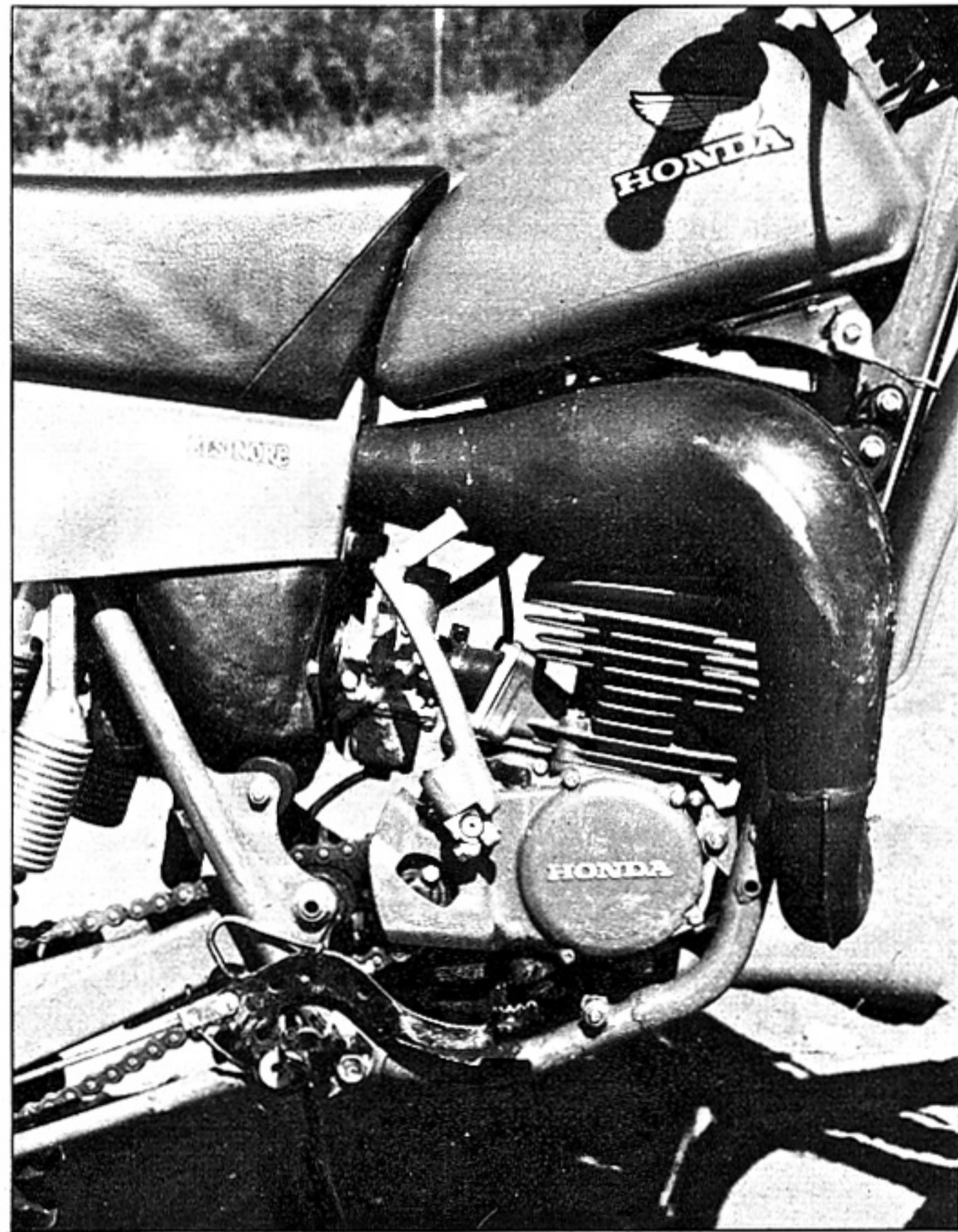
Gas tank material is now plastic for better durability, and a new expansion chamber has been welded into the pipe to suit the center-port cylinder.
