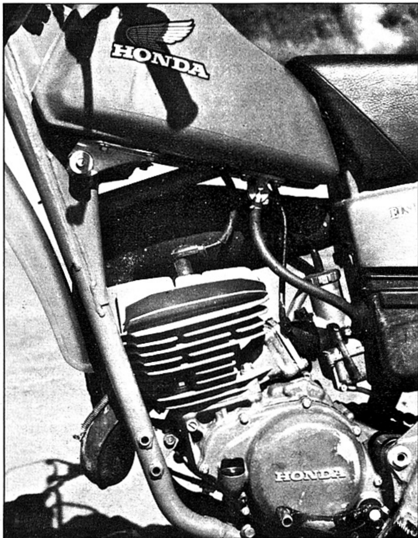
The factory went out to the works bikes and took off a center-port cylinder for this year's 125, along with more fin area.
