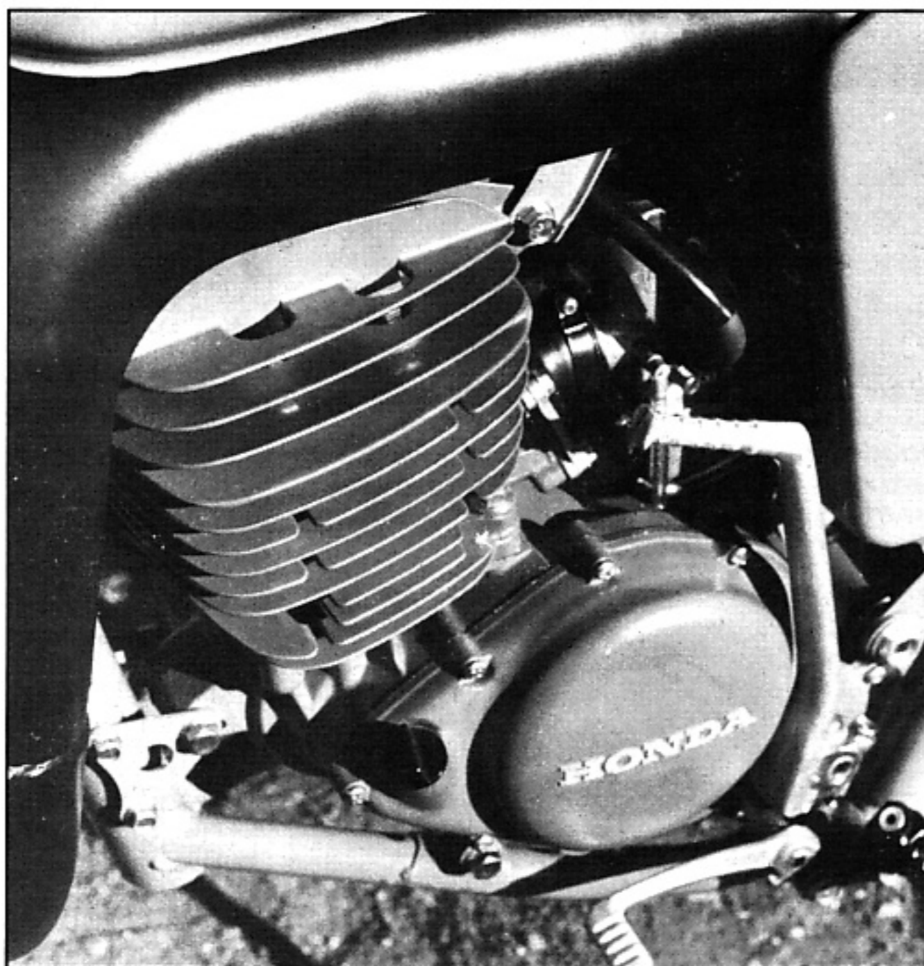
(ABOVE) Engine compartment is packed without being crowded. Placement of parts shows much thought. Head steady at rear of motor is important. Keep it tight.
