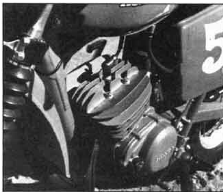
Engine looks almost tiny in the roomy frame. Less carb, actual weight of bright red motor is under 40 pounds. Finning looks on the smallish side.
