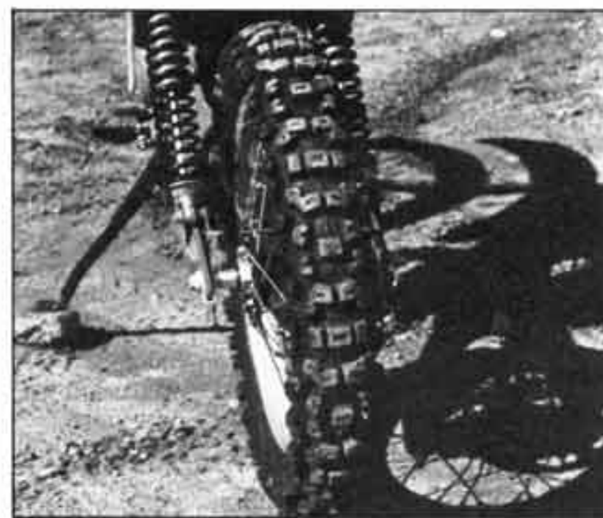
Claw Action tires are a Honda/Bridgestone joint effort. While straight-line traction is excellent, the tires roll badly under heavy side loads.
