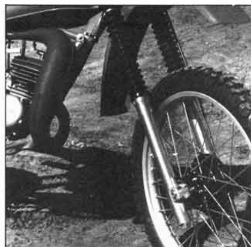
Forks had 11 inches of travel and did a decent job on the bumps. New caps on axle are four-bolt pattern and very strong. This should help keep fork flex to a minimum.
