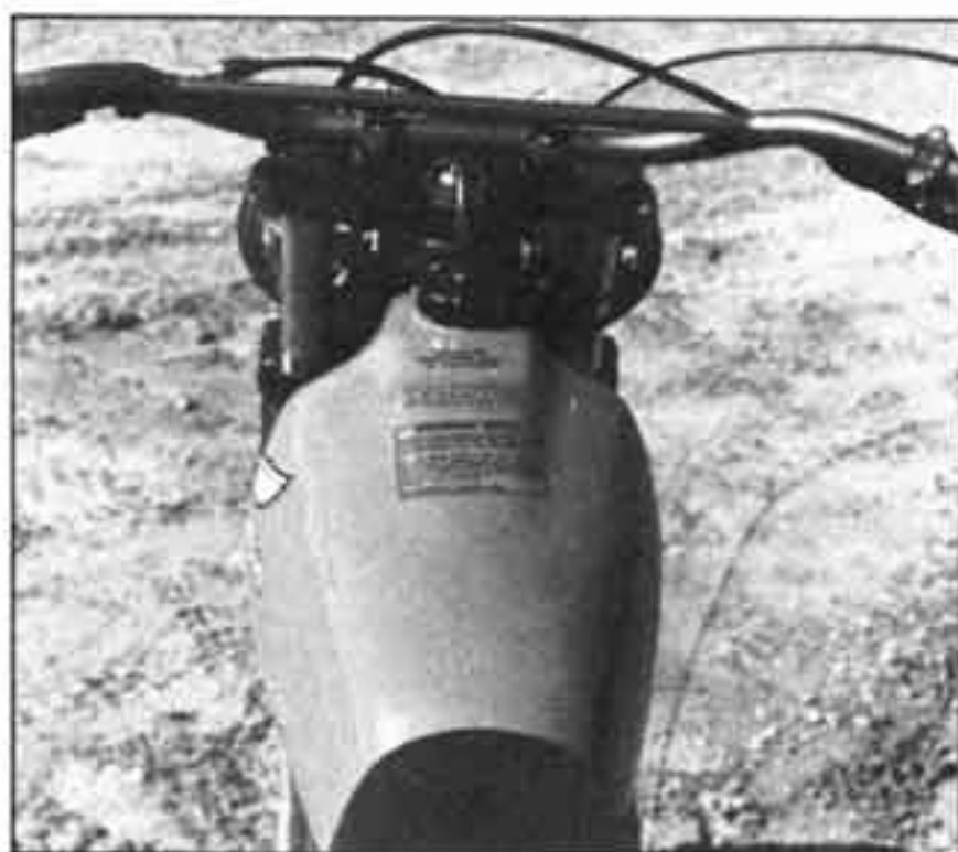
As per usual Honda practice, the CR125R is loaded with decals warning the rider of just about everything. Bars had an odd feel, being high and angled sharply forward. When riders rotated them back for greater comfort, the ends then sloped down like a divining rod.
