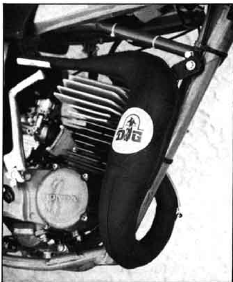
DG pipe is formed from die-stamping.
