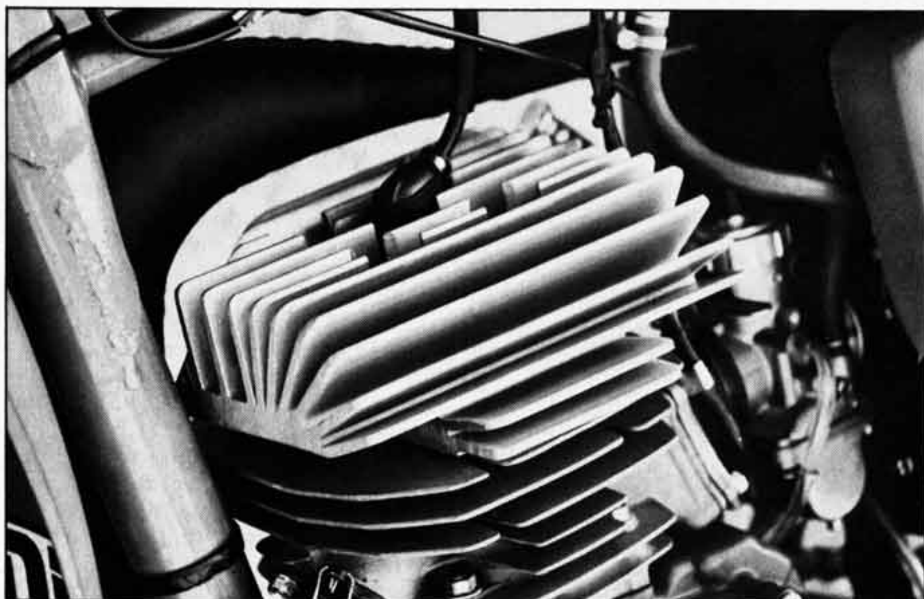
Aluminum head runs up to 100° cooler than stock.
