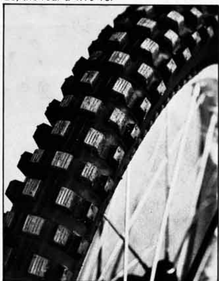
New IRC tires work well. The front is a 3.00-23, the rear a 4.10-18.
