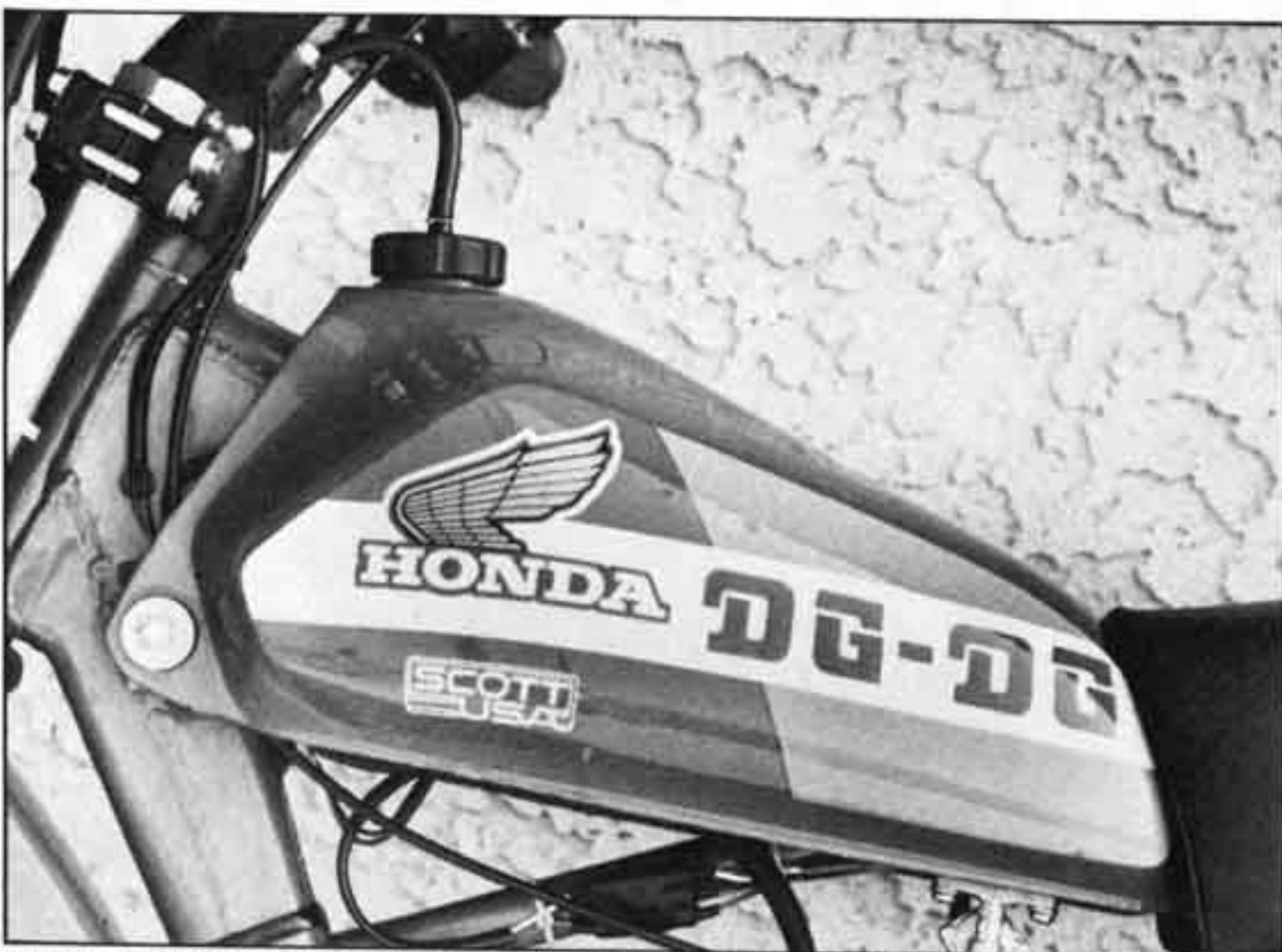
Stock tank is protected from abrasion by DG decals.
