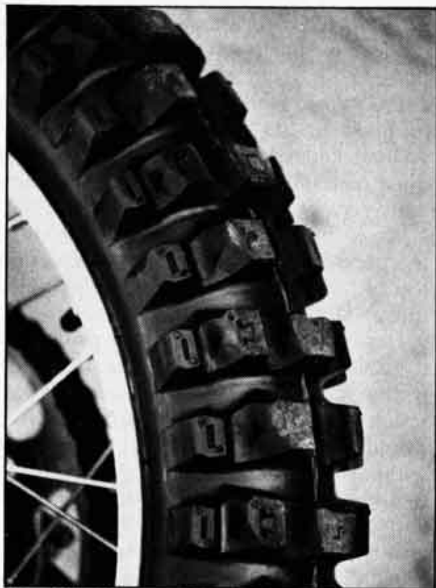
New IRC tires work well. The front is a 3.00-23, the rear a 4.10-18.
