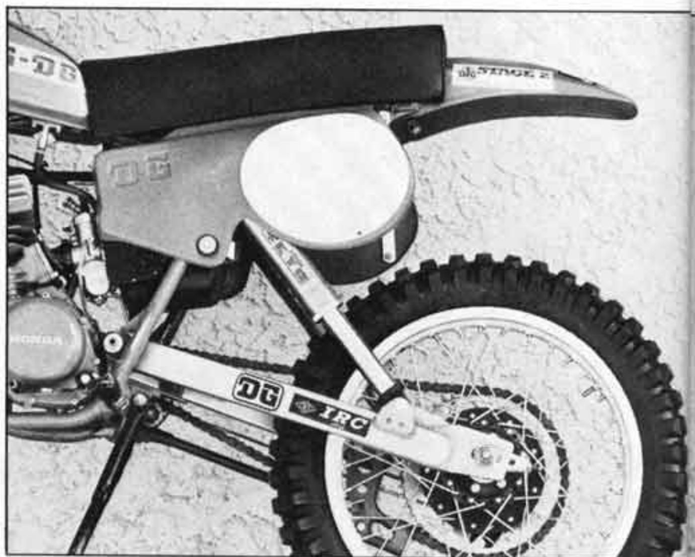
Aluminum swing arm is 1 in. longer than stock. KYB F Series air spring shocks are adjustable and rebuildable.
