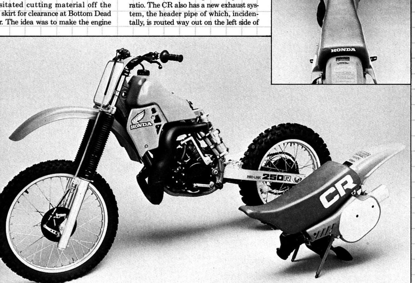
With the removal of three bolts and two clamps, the tail of the Honda detaches with the seat, airbox and silencer
