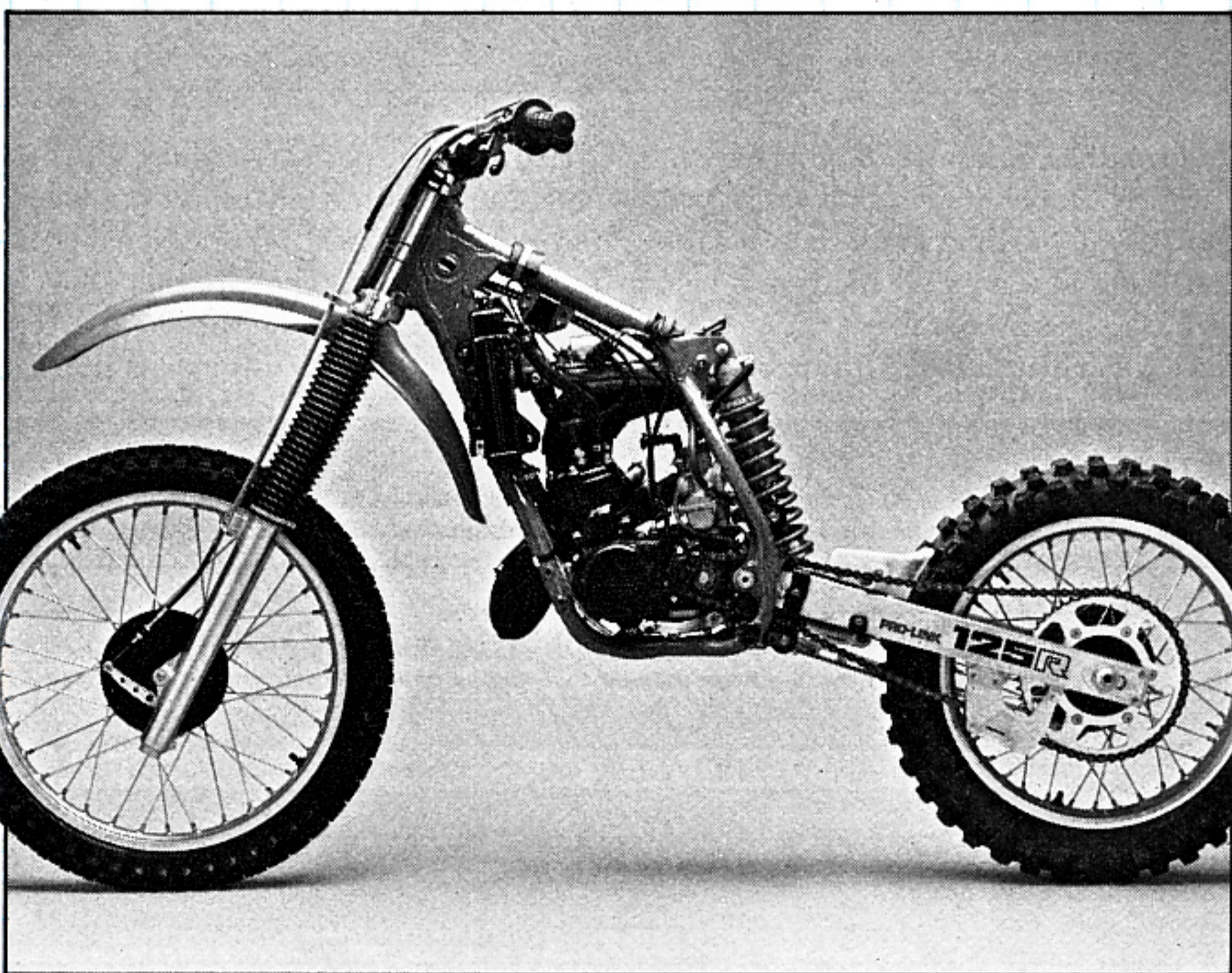
Rebound-damping screw has 30 clicks But only the first 20 have any effect.
