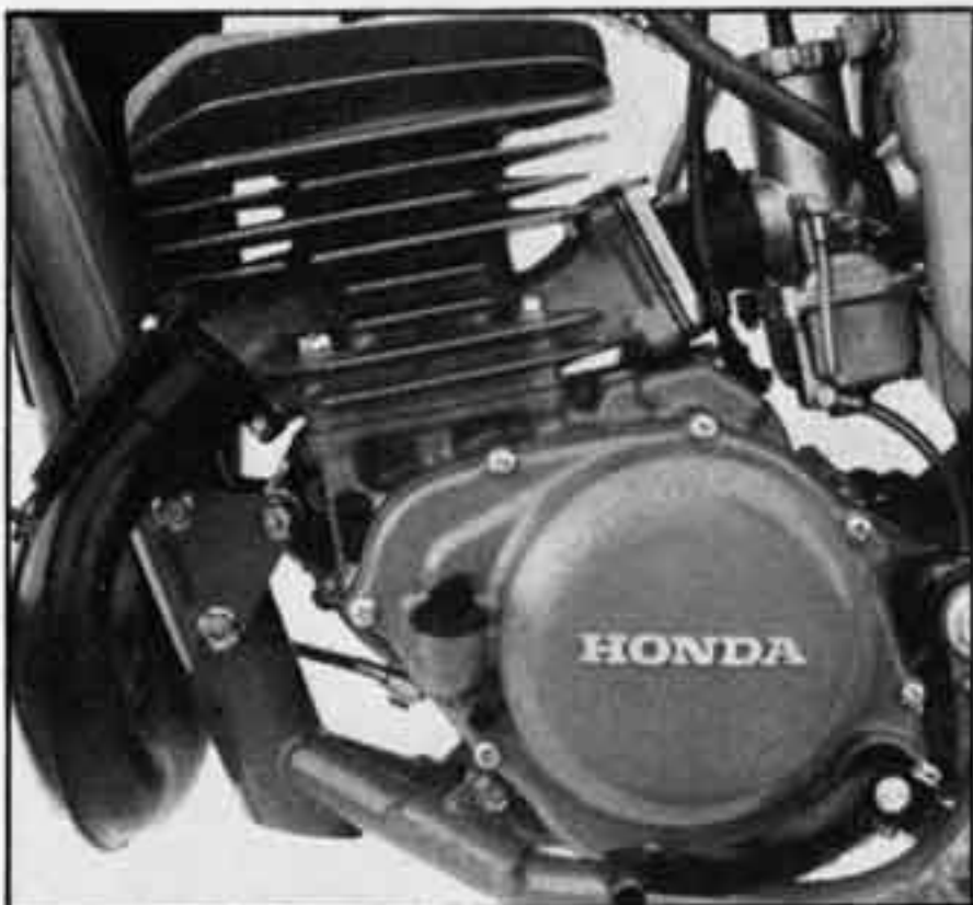
Light, unusually short six-speed engine Not a wasted scrap of alloy anywhere.
