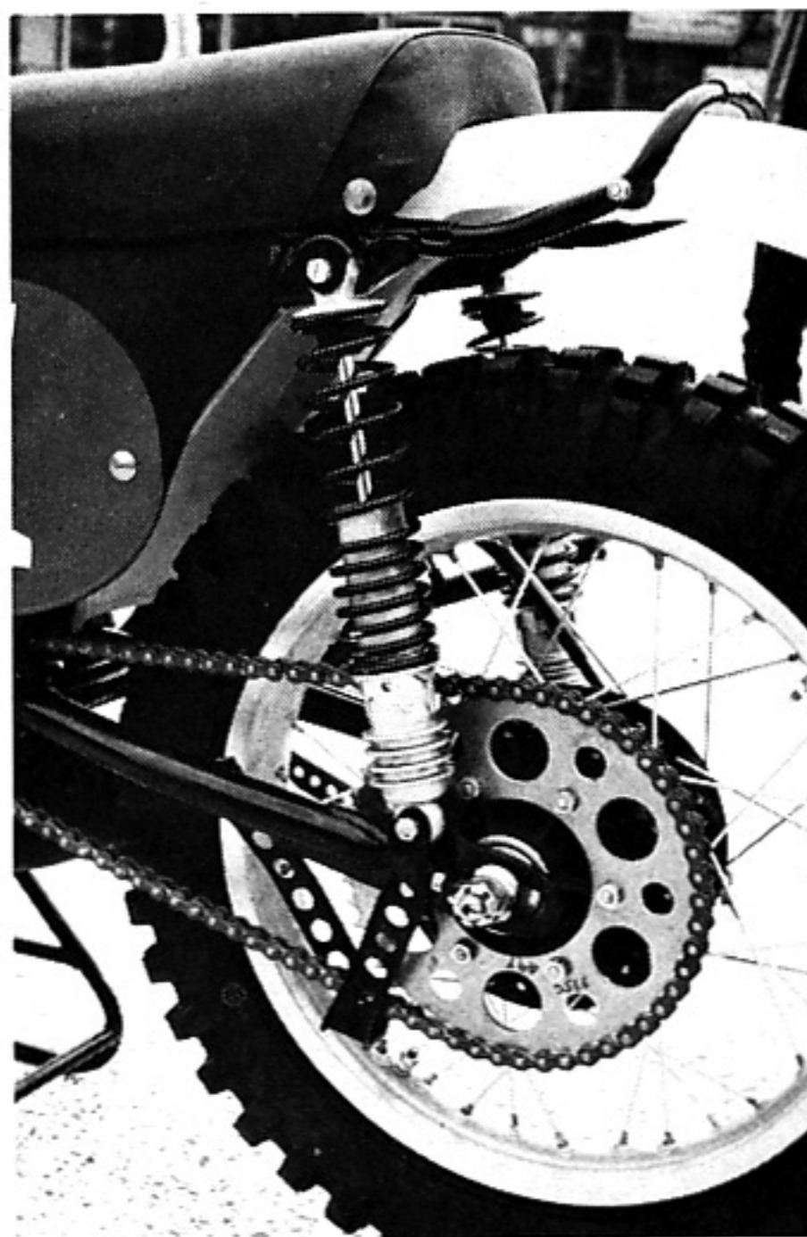
The rear dampers use a progressively wound spring of few turns. We can't quite figure out what those fins around the bottom of the shocks are for. Note the extensive use of lightning holes.
