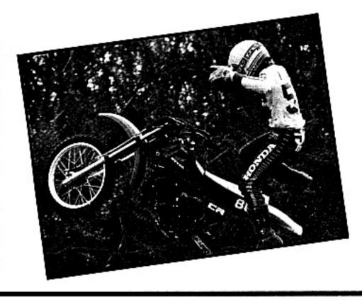
Honda CR's Pro-Link has a remote-reservoir shock with preload and damping adjustments. Up front, a 31mm air-assisted fork has tubes which slide on Honda's Syntallic bushings. Spokes with increased diameter link the Honda's new rims and hubs.
