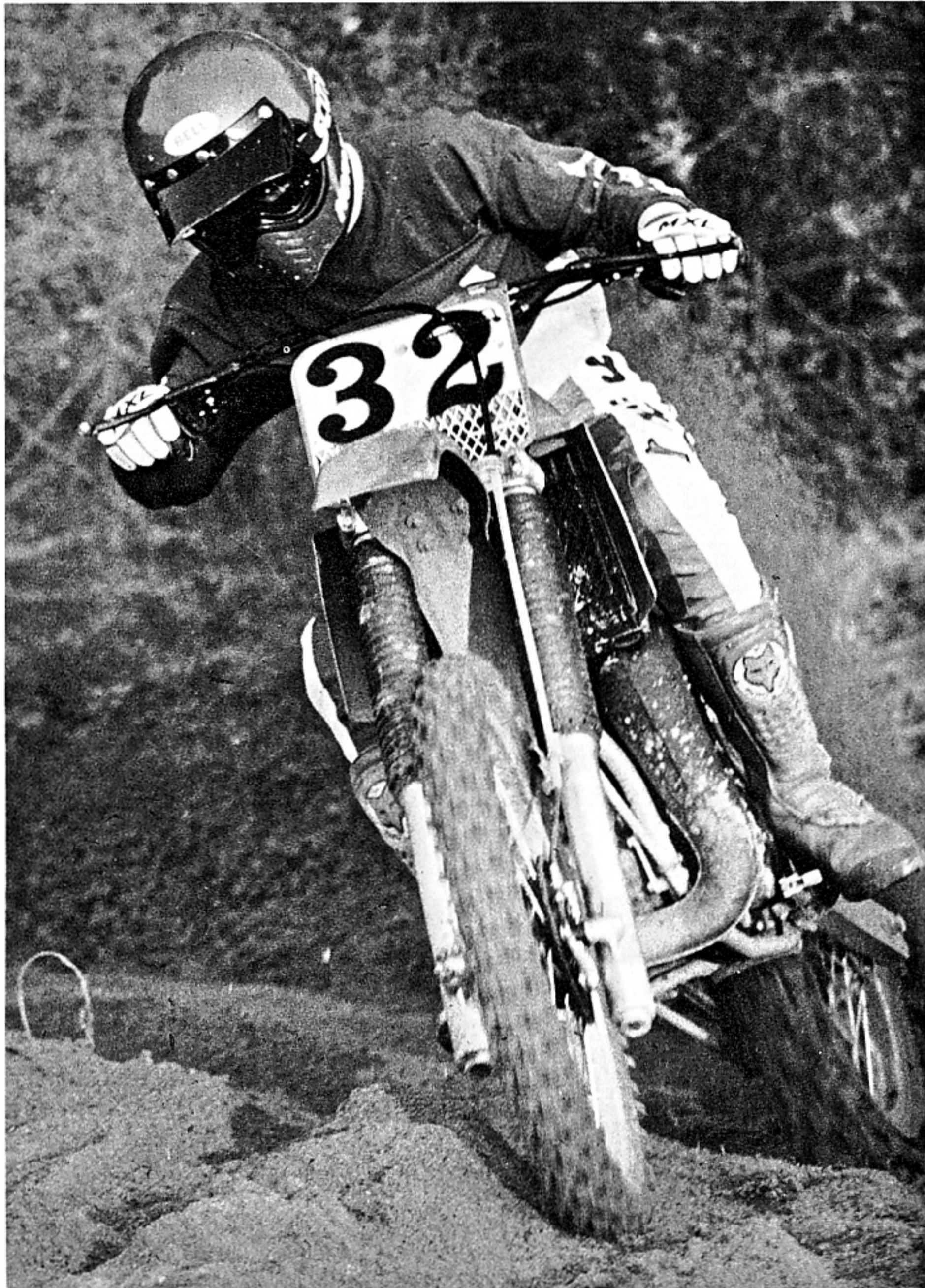
Refinements abound: contoured shift lever stays out of your boot's way, a new brake spring works well . . . the swing arm mounts the axle more solidly than before, and the brake arm is now aluminum.
