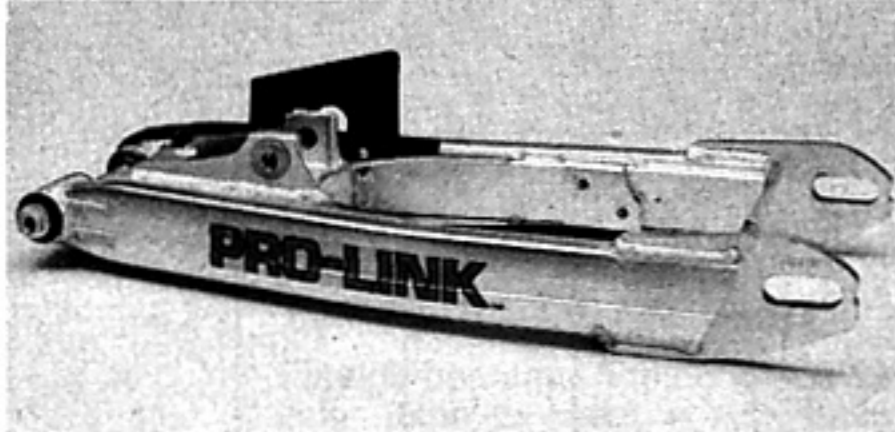
A straightforward system: as the swing arm rises, it compresses the shock via a pivoting linkage.
