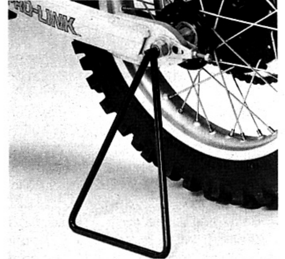
To eliminate any unnecessary items attached to the CR, Honda uses a stand which plugs into the axle.
