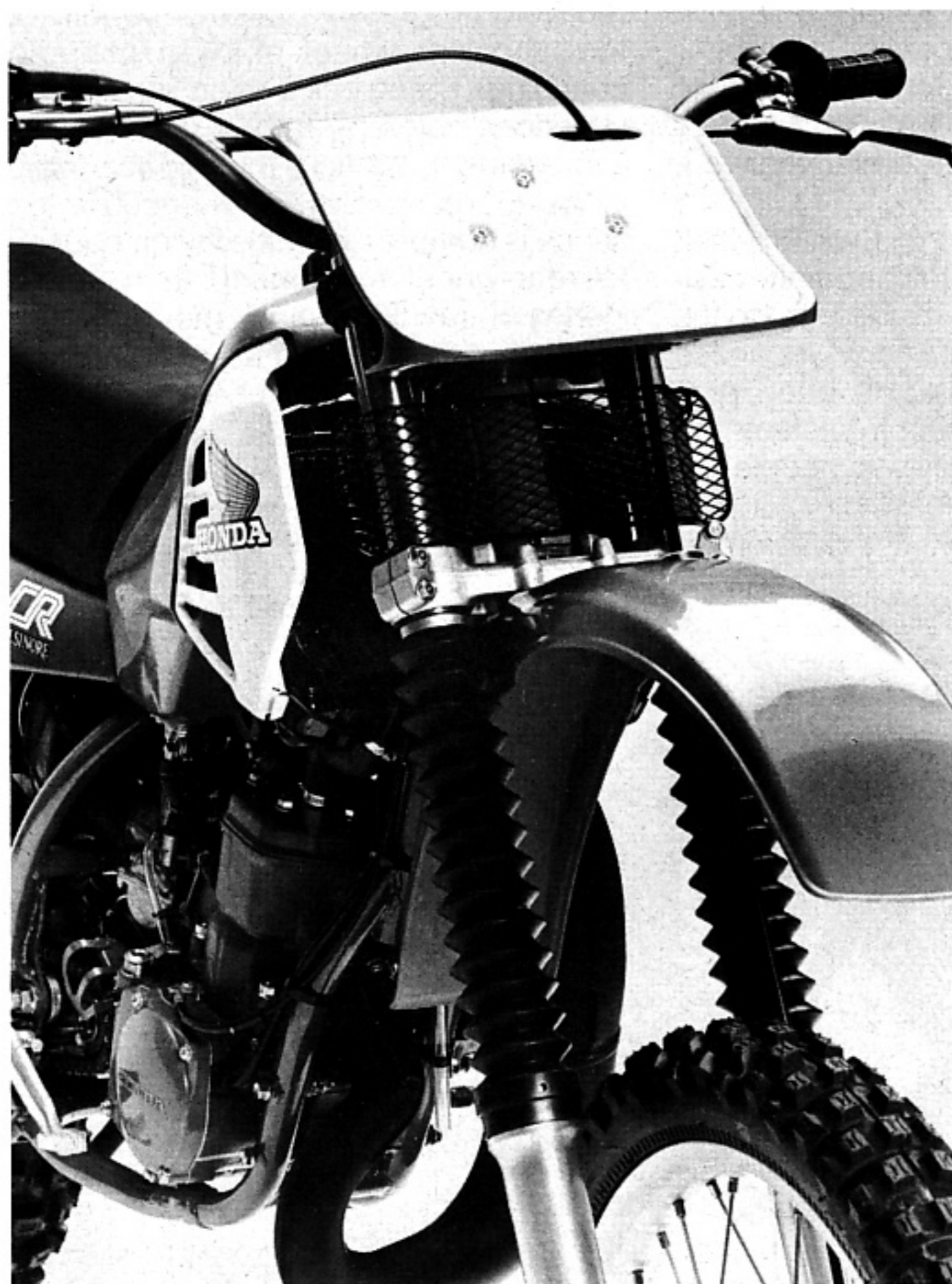
Fork-mounted screen and radiator-mounted screens protect the front of the radiators; shields guard the sides. New frame allows the center-port engine.
