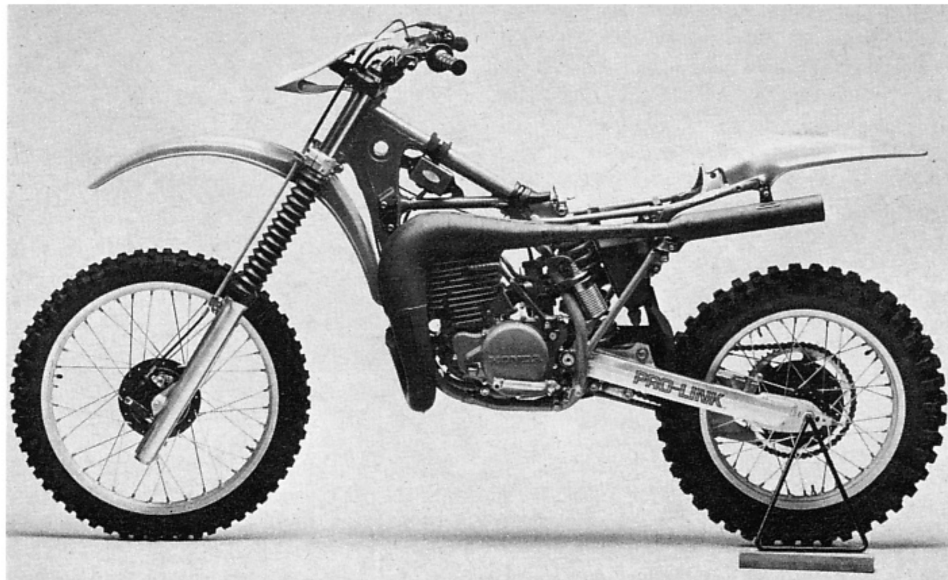
Shock location requires the airbox passage to skirt the right while the reservoir mounts on the left side.
