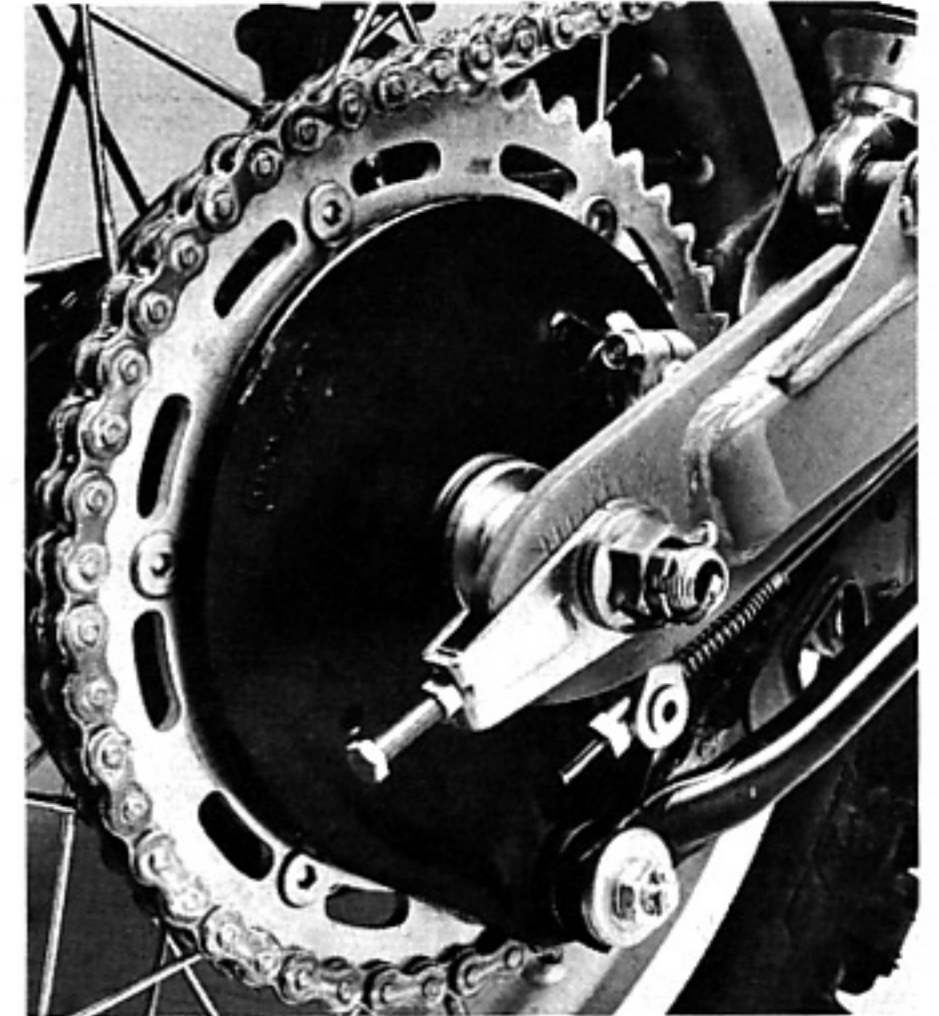
Titanium chain adjuster, aluminum rear brake arm, full-floating torque arm, specially machined chain guide and strong, thick and heavy swing arm all highlight the RC's rear end. The same pieces on the production CR are stamped or drawn from mild steel.
