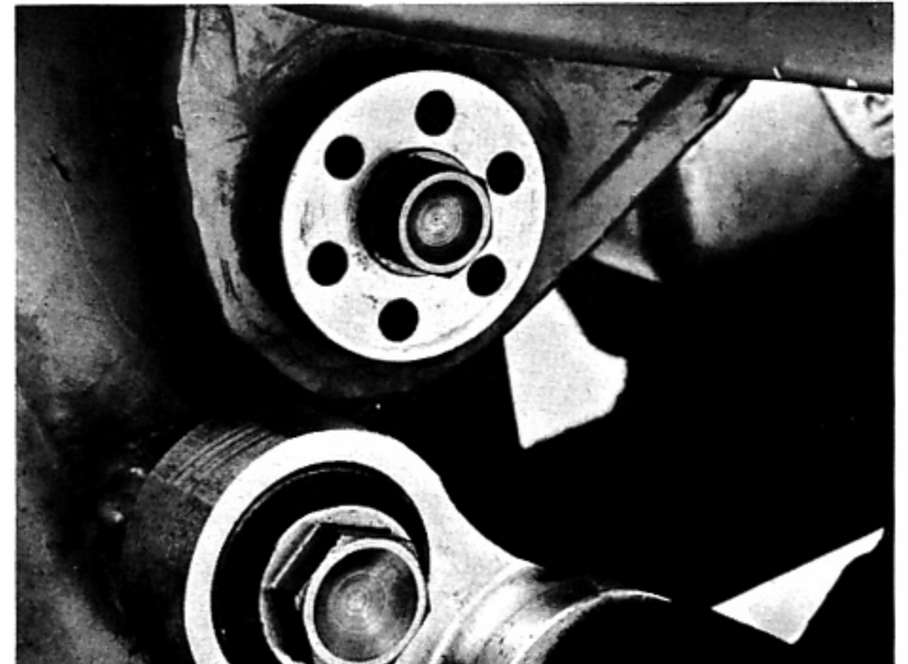
A quarter-ounce aluminum washer is drilled to further lighten the piece.
