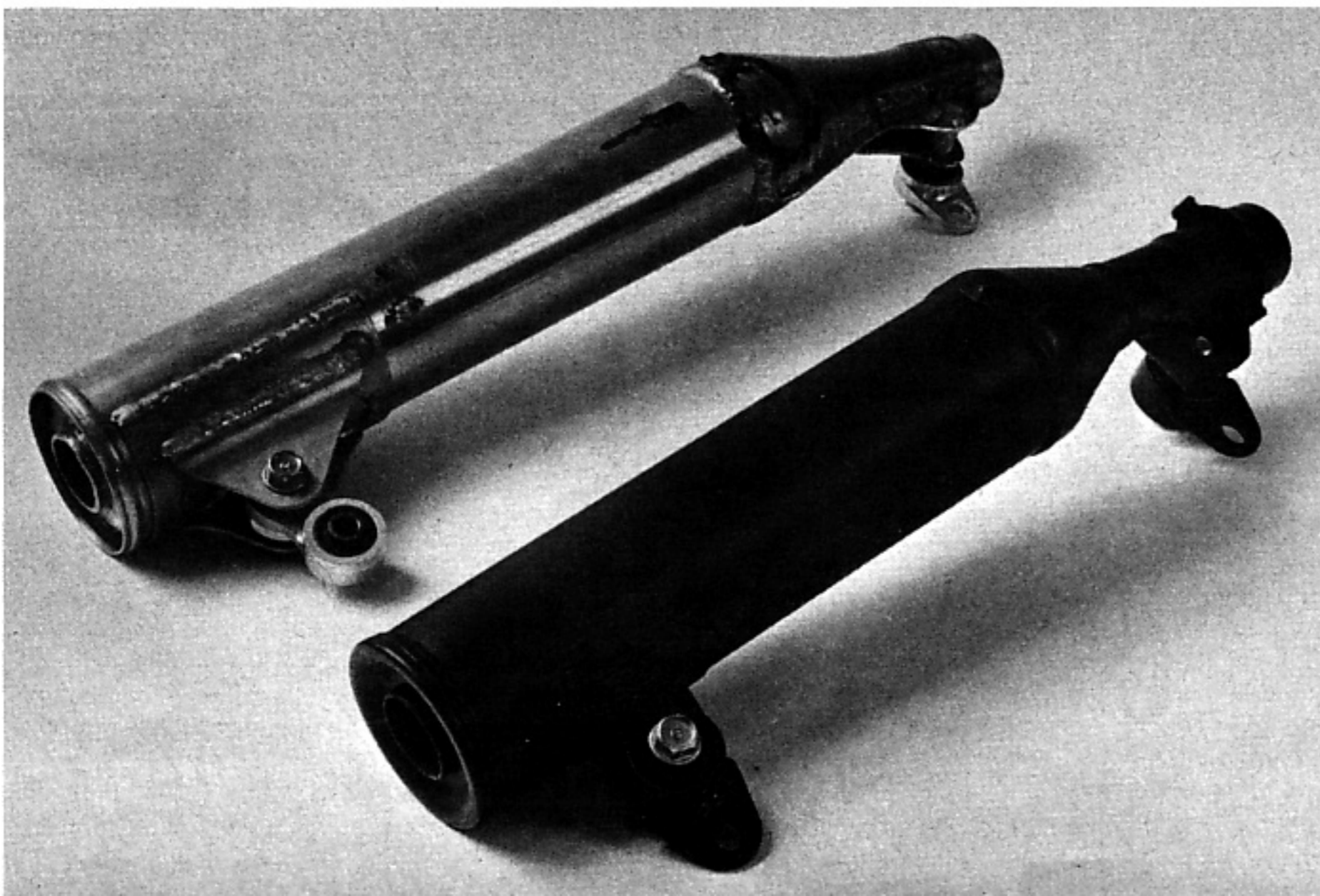
Aluminum RC silencer is the same size as black steel stock model but a whopping two pounds lighter.
