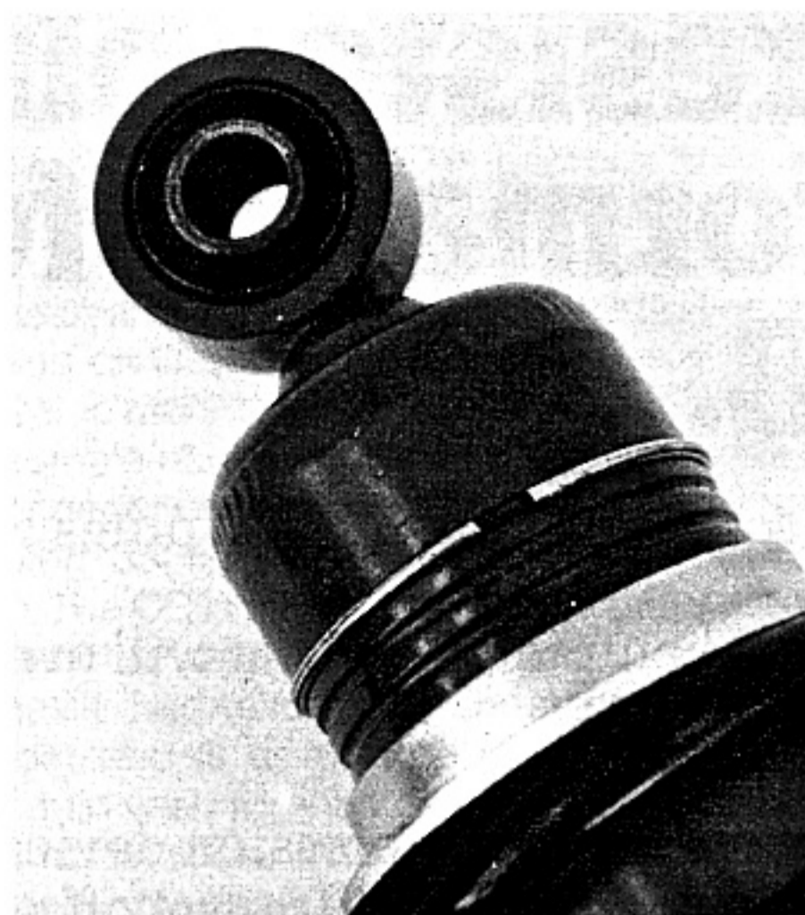
Frail-looking clips adjust the rear spring preload and are hard to use when the shock bodies are dirty.
