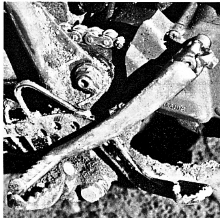
. . . but the right peg was bent back by a rock and caught the kickstart arm the next time it was used.
