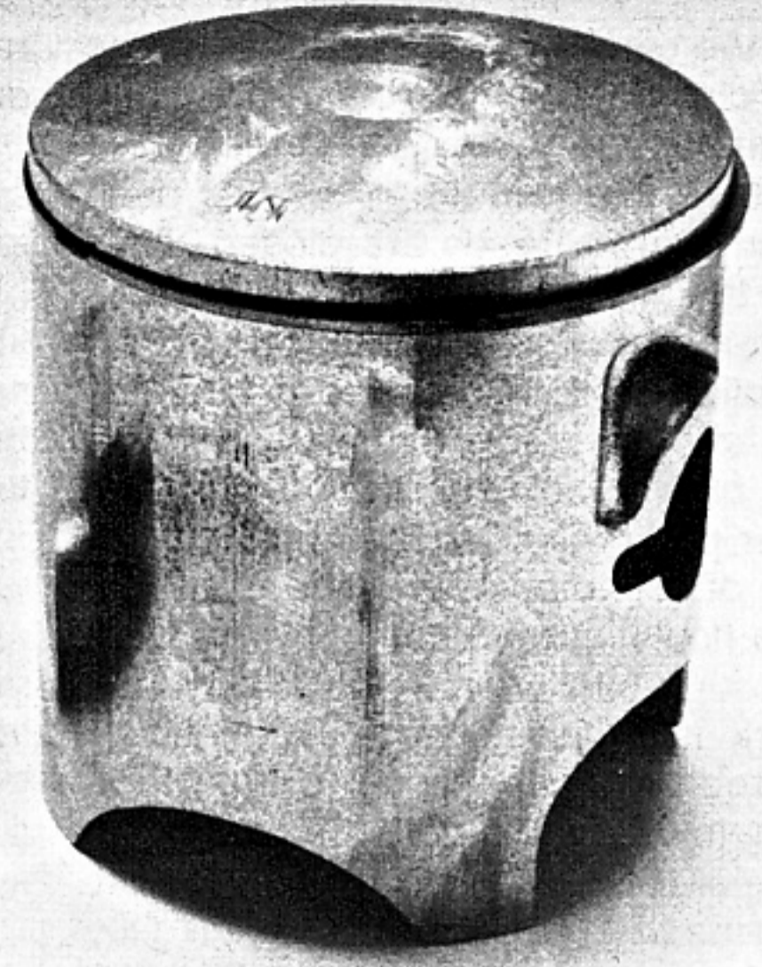
Standard motocross technology calls for a one-ring aluminum piston, hardened-steel wrist pin and steel-caged needle bearings.
