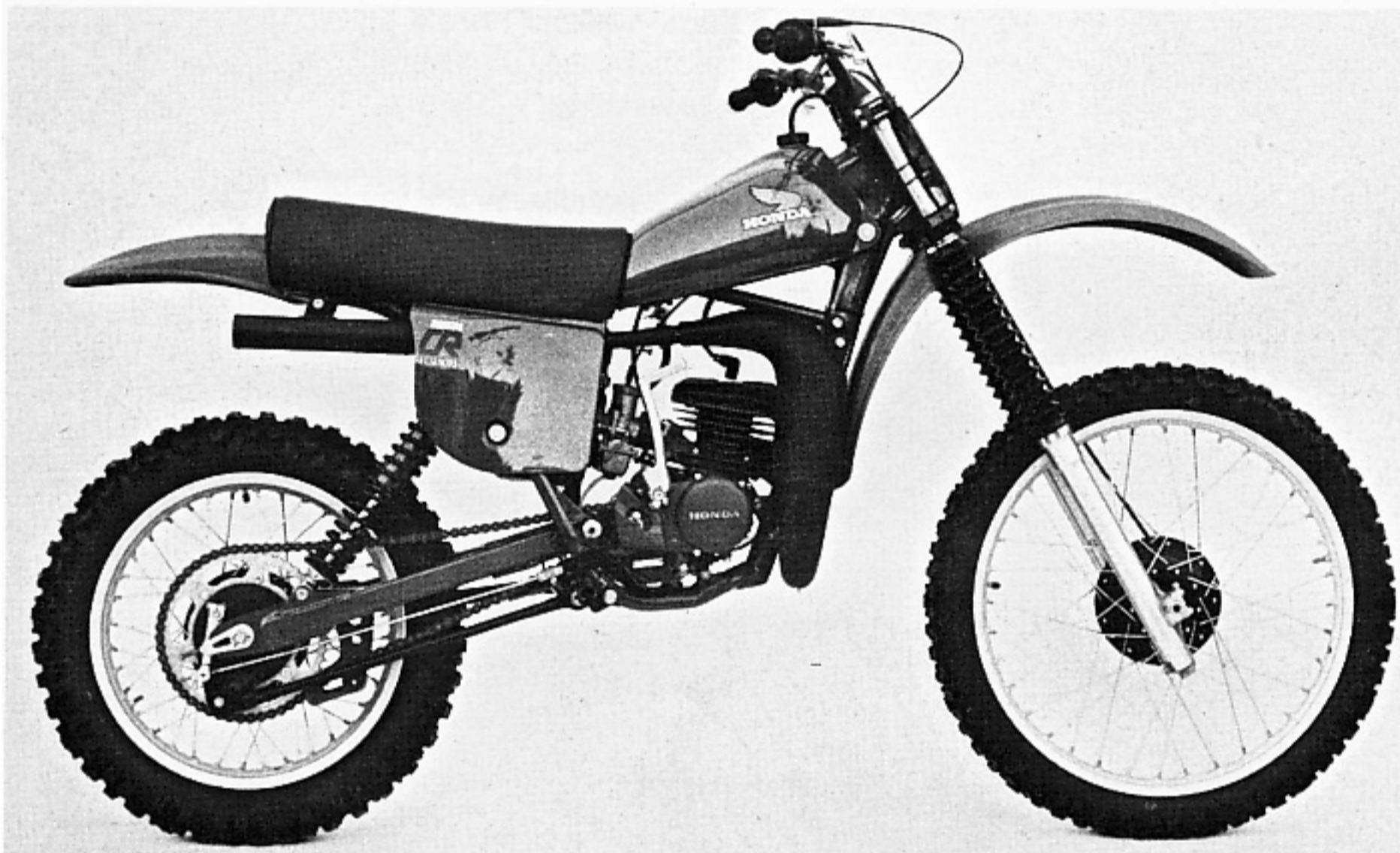
Aluminum engine cases are cored for lightness, and oil cups (right) ensure bearing longevity. Shifting mechanism is tried-and-true Elsinore.
