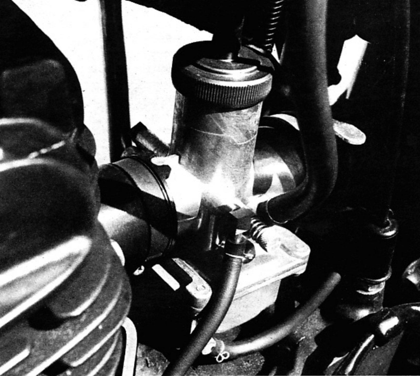
MT-125 has 24mm Keihin; the alloy carb has closed-cell foam floats.
