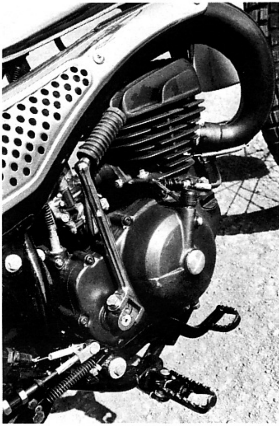
Some parts of the MT-125 show serious intent: an out-of-the-way brake lever and serrated spring-loaded 45-degree pegs. The lighting equipment is all QD. The fixture is a zener-diode in a plug. Neat!
