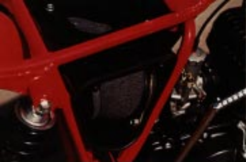
Easily accessible CR-125M air filter element is protected against dust and water.
