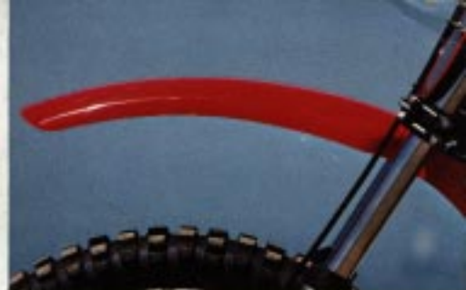
Both bikes have tough, flexible plastic fenders which have been redesigned for better rider protection.
