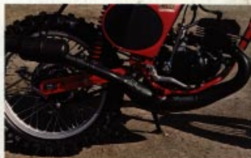
Redesigned CR-125M engine provides more horsepower. Larger cooling fins added for better heat dissipation.
