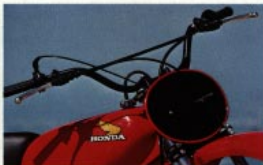
Wide flat black handlebars with malleable control levers. Front and side number plates standard.
