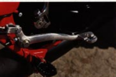
Elsinores have an aluminum brake pedal lever that is notched for sure footing and tucked in out of the way.
