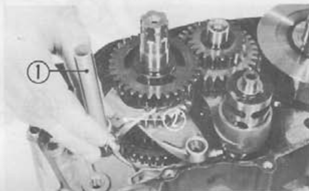
Fig. 4-77 ① Gearshift fork shaft ② Left gearshift fork
