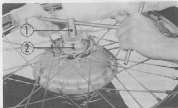
Fig. 5-4 ① Front wheel axle ② Speedometer gear box
