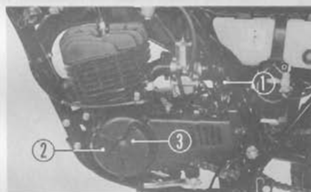
Fig. 4-32 ① Wire harness connector ② Left crankcase cover ③ Generator rotor cover
