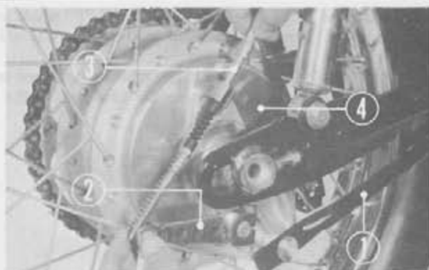
Fig. 5-15 ① Rear brake stopper arm ② Rear brake arm ③ Rear brake cable ④ Brake panel
