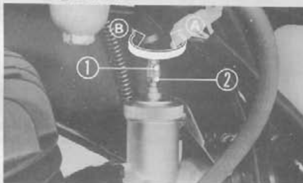
Fig. 3-3 ① Adjusting screw ② Lock nut
