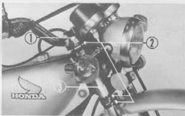
Fig. 5-36 ① Fork bolt ③ Front fork ② Front fork tightening bolts
