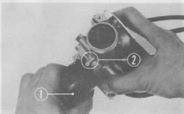
Fig. 4-101 ① Inlet pipe ② Recess in inlet pipe
