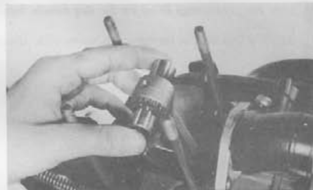
Fig. 4-24 Checking connecting rod small end bearing for looseness
