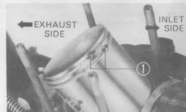
Fig. 4-26 ① Piston ring stopper
