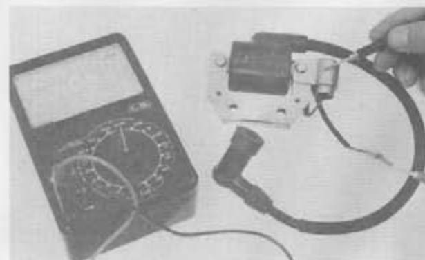
Fig. 6-13 Checking condenser for condition
