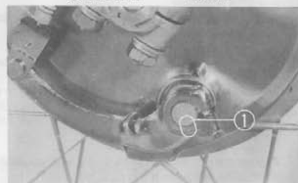
Fig. 3-19 ① Punch mark on serration
