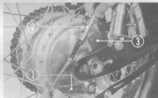
Fig. 5-25 ① Rear brake arm ③ Rear brake panel ② Rear brake cable
