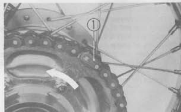
Fig. 4-7 ① Master link retaining
