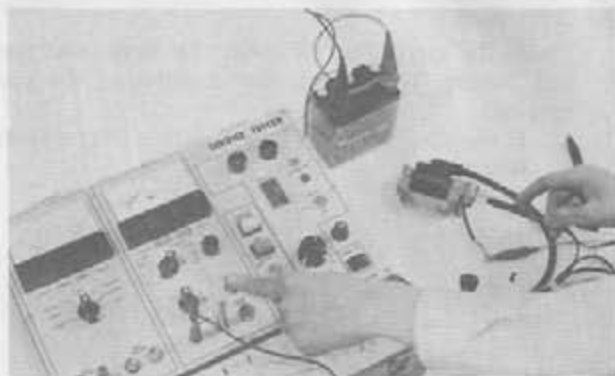
Fig. 6-10 Ignition coil continuity test
