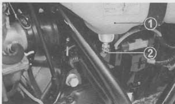
Fig. K1-4 (1) Oil tank (2) Oil tube protector
