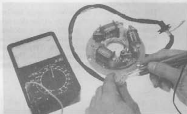
Fig. 6-4 Stator continuity test
