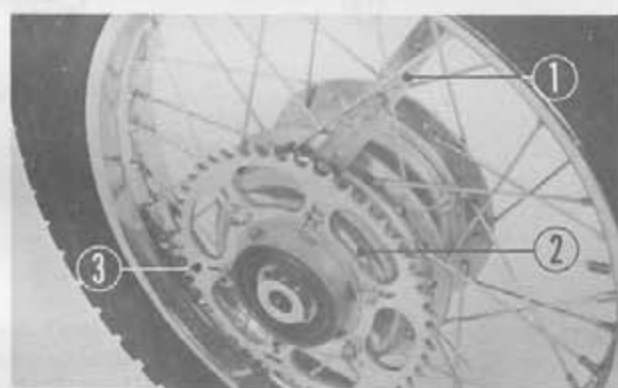
Fig. 5-17 ① Wood block ③ Driven sprocket ② Driven flange
