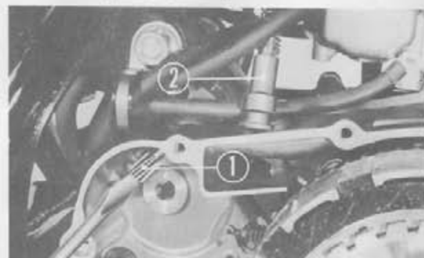
Fig. 4-55 ① Tachometer drive gear ② Tachometer cable
