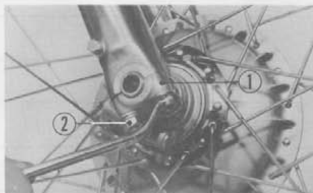
Fig. 5-3 ① Front axle holder ② Axle holder tightening nuts
