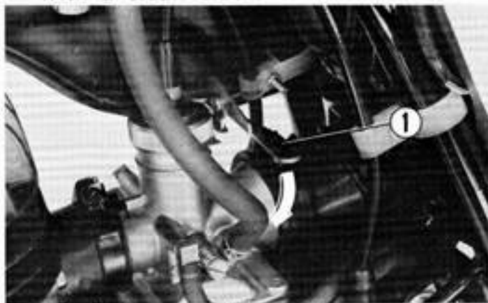
① Fuel mixture enrichment lever
