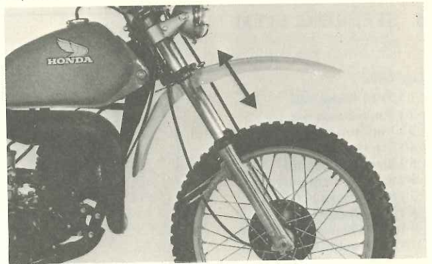
Fig. 4-56 Checking movement of front fork
