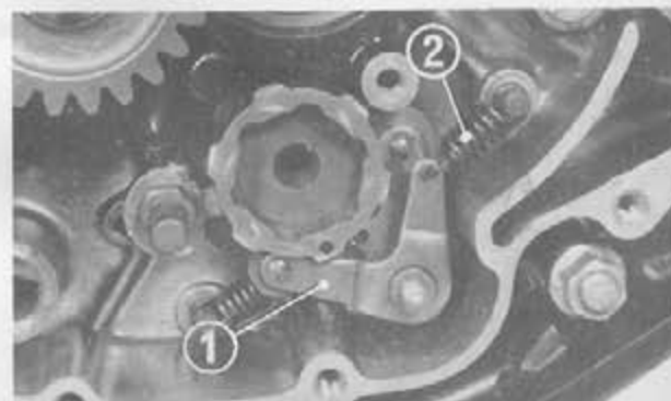
Fig. 3-47 (1) Neutral stopper arm (2) Neutral stopper arm spring
