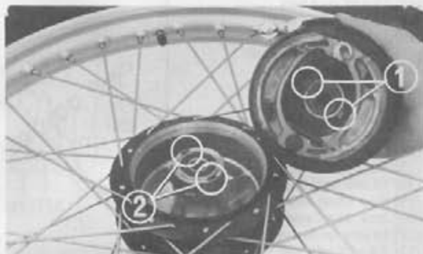
Fig. 4-9 (1) Lugs of speedometer gear (2) Groove in the wheel hub
