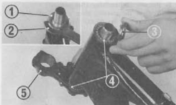
Fig. 4-61 (1) 45 mm pin wrench (2) Steering head top thread (3) Top cone race (4) # 6 steel balls (5) Steering stem
