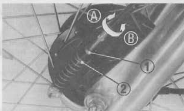
Fig. 2-32 (1) Lock nut (2) Front brake adjusting nut
