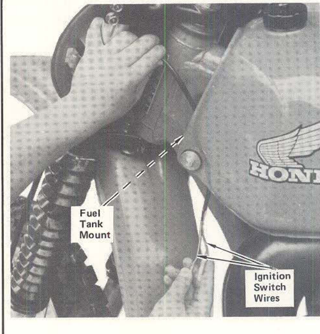
STEP 53 —Route ignition switch wires above left fuel tank mount between fuel tank and frame. Press wires into space between fuel tank and frame.
