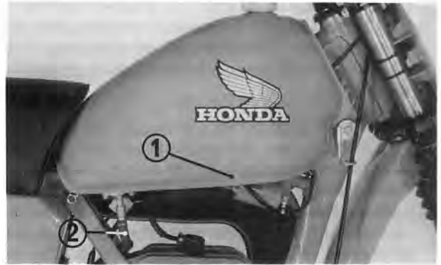
Fig. 2-46 (1) Fuel tank (2) Fuel line
