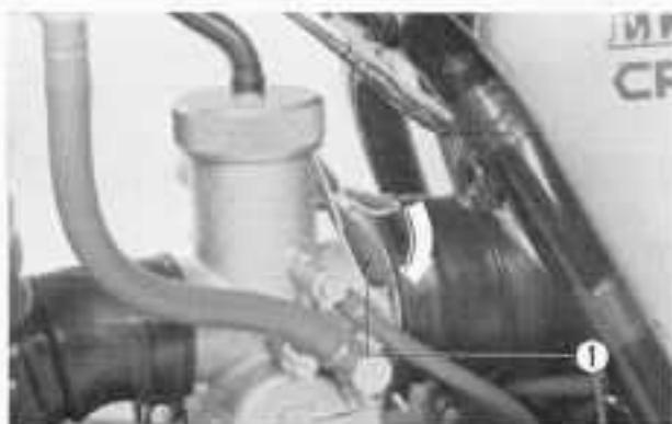
Fig. 1-4 (1) Fuel mixture enrichment lever
