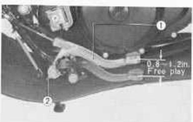
Fig. 2-31 ① Rear brake pedal
