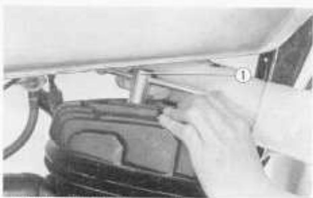
Fig. 2-6 ① Spark plug wrench
