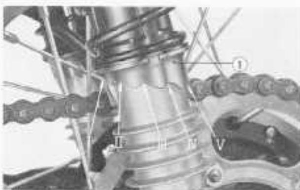
Fig. 2-25 ① Spring adjuster
