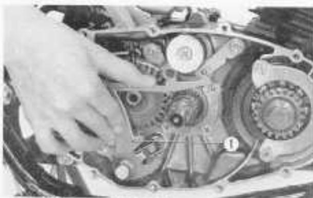
Fig. 3-20 ① Gearshift spindle
