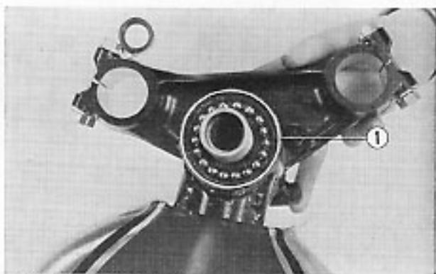
Fig. 4-5 ① Steel balls
